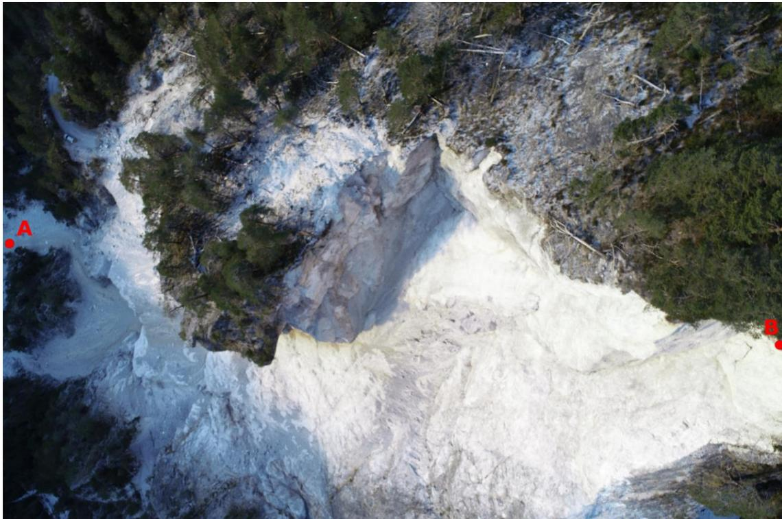
**Figure 3.** Extreme height differences in a steep terrain result in a varying GSD within the vertical image (~0.5 cm in point A and ~7.9 cm in point B).
