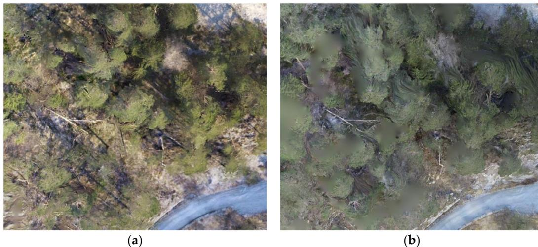
**Figure 18.** Inserts of orthophoto with 5-cm resolution: (a) from vertical images and (b) from oblique images.
