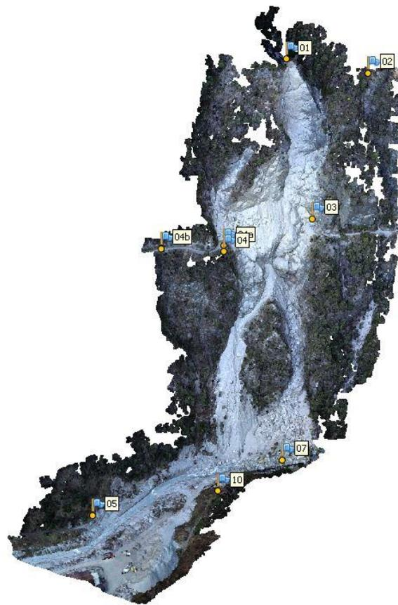
**Figure 10.** Distribution of GCPs (shown on the dense point cloud).
