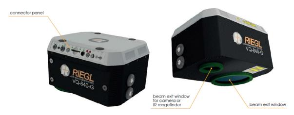
**Figure 1.** Computer Aided Design rendering of the VQ-840-G laser scanning system in basic configuration. The electrical and data interfaces are shown on the left hand side while the apertures for the green laser scanner and the camera at the bottom of the unit are shown on the right hand side.
