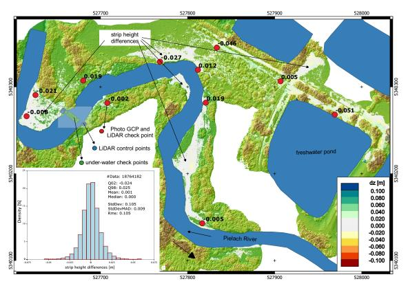
**Figure 9.** Color coded mosaic of strip height differences, background: LiDAR DSM (color coded elevation map superimposed with shaded relief map), lower left: histogram of height differences in smooth surface areas, lower right: color bar for strip differences.
