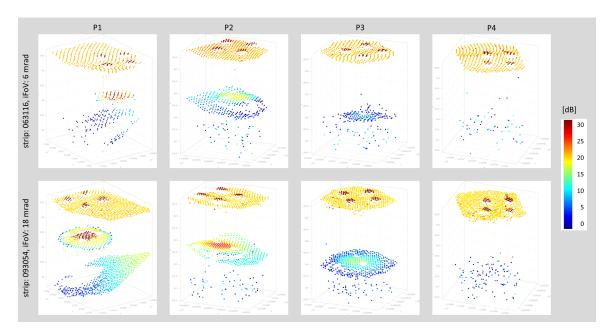
**Figure 12.** Perspective view of 3D point points of lowered metal plates P1-P4 colored by signal amplitude [dB]. upper row: strip 063116, iFoV: 6 mrad, lower row: strip 093054, iFoV: 18 mrad.
