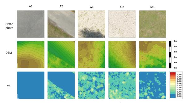
**Figure 8.** Visualization of measurement noise for selected  $5 \times 5 \text{ m}^2$  surface patches; A1: asphalt, A2: asphalt and grass, G1/G2: gravel bank, M1: meadow; first row: digital orthophoto, second row: color coded height map superimposed with 1 cm contour lines, third row: color coded map of local surface roughness (i.e.,  $\sigma_0$  [m]).
