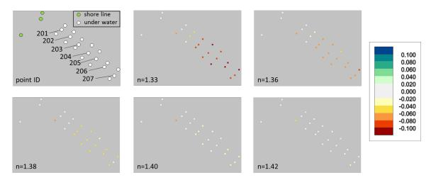
**Figure 10.** Color coded point-to-plane distances [m] between check points and LiDAR derived planes, run-time correction based on refraction coefficients ranging from n = 1.33 to n = 1.42.
