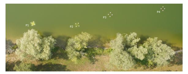
**Figure 5.** The  $1 \times 1$  m<sup>2</sup> plates (P1–P4) floating in pond FP1 for evaluation of depth performance; camera:  $\alpha$ 7R; acquisition: day 1; depth of plate from left to right: 1.1 m, 1.9 m, 2.6 m, 3.1 m.
