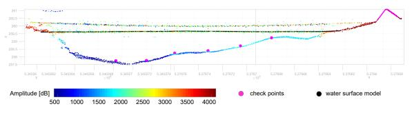
**Figure 11.** Vertical section of refraction corrected 3D point cloud (n = 1.36) of strip 105334 colored by signal amplitude; larger magenta dots: checkpoints, black: modelled water surface.
