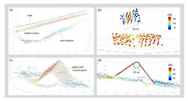
**Figure 14.** Empirical assessment of spatial resolution; top row: rope spanned across river, bottom row: gable roof shaped control patch; (**a**–**c**) perspective view of 3D point cloud; (**d**) vertical section; points colored by signal amplitude [dB].
