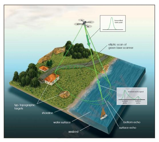
**Figure 2.** Visualisation of the VQ-840-G mounted on a drone in operation. The scan pattern on the ground is indicated by the green ellipse. The inserts show typical pulse shapes of the outgoing laser pulse and the echo return when measuring into the water.
