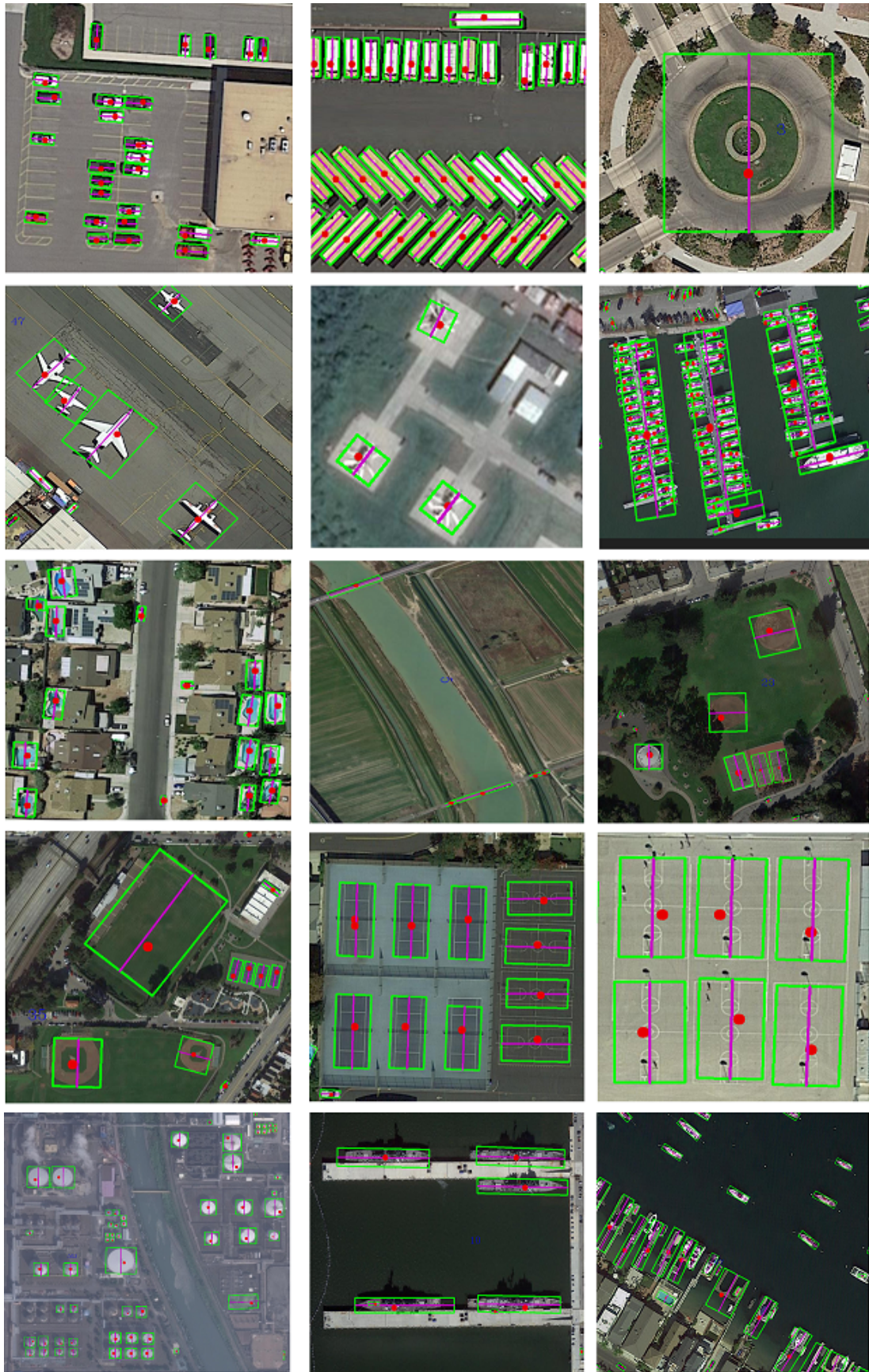
Figure 4. Detection results of our method on DOTA. Red points stand the mapping points from feature maps, which predict the axis and width. Pink lines stand the axes detection.
