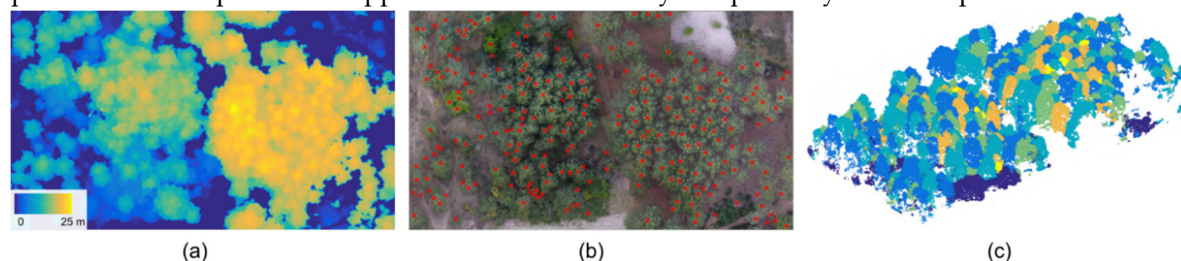
Figure 2. Example of an individual tree crown detection and delineation approach using: (a) a canopy height model; (b) identified treetops using local maxima; and (c) tree crown delineation using watershed transform.
