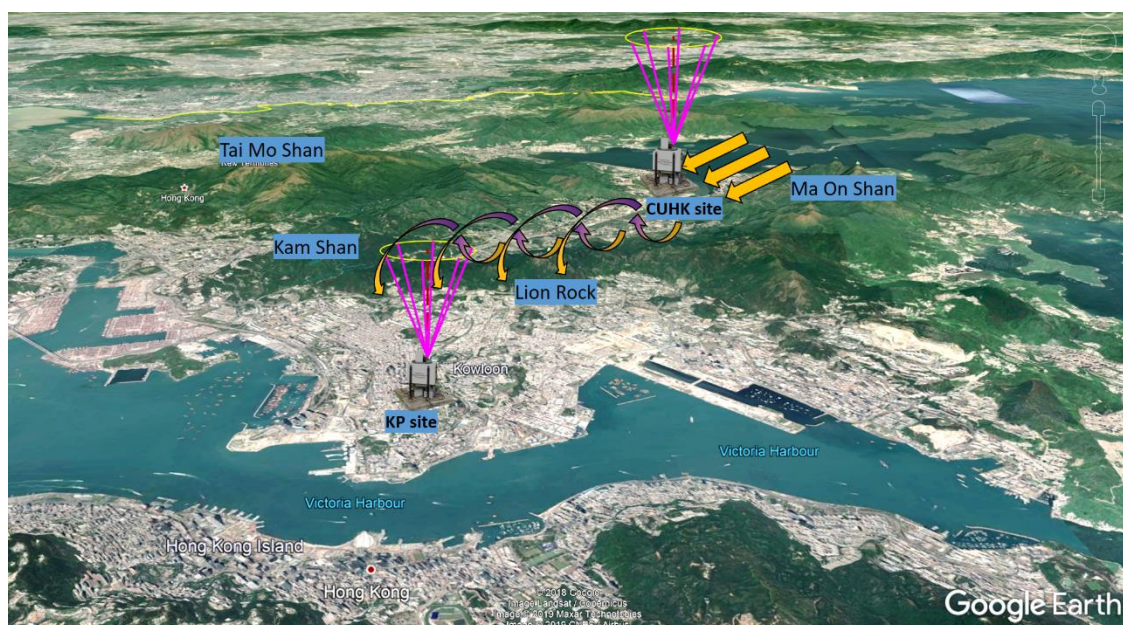
Figure 1. Locations of the two LiDAR sites (CUHK and KP), topography near the CUHK site, and schematic of the upslope and downslope winds. The arrows refer to wind direction. The arrow colors refer to altitude: orange: lower altitude; purple: higher altitude. This CUHK site is surrounded by mountains, including Ma On Shan ( \approx 700 m), Lion Rock ( \approx 500 m), Kam Shan ( \approx 370 m), and Tai Mo Shan ( \approx 957 m). The figure was built on a map obtained from Google Earth, earth.google.com/web/ .
