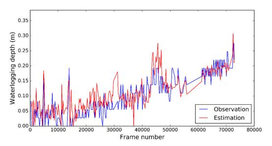
**Figure 9.** The waterlogging depths calculated based on the heights of the reference objects detected manually (i.e., observations) and the waterlogging depths calculated based on the heights of the reference objects detected by the SSD (i.e., estimations).
