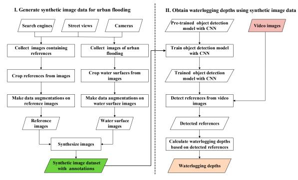
**Figure 1.** Flow chart of the proposed method and its further application in obtaining waterlogging depths.
