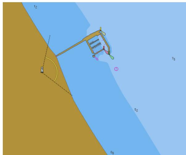
Figure 5. Bathymetric chart of the marina area in Sopot made on the basis of official electronic navigational chart (ENC) data.
