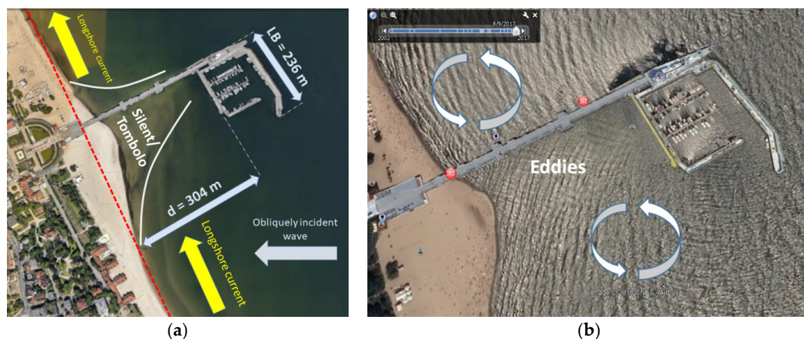
Figure 1. The nature of the phenomenon that causes the formation of the tombolo effect (a), and the wavy surface of the sea in varying directions resulting from the diffraction of waves around the marina breakwater in Sopot (b).
