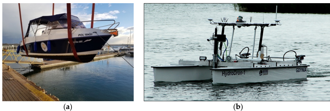
Figure 7. Hydrographic vessel with a draft of 30 cm (a) and unmanned surface vehicle (USV) designed for coastal measurements (b).
