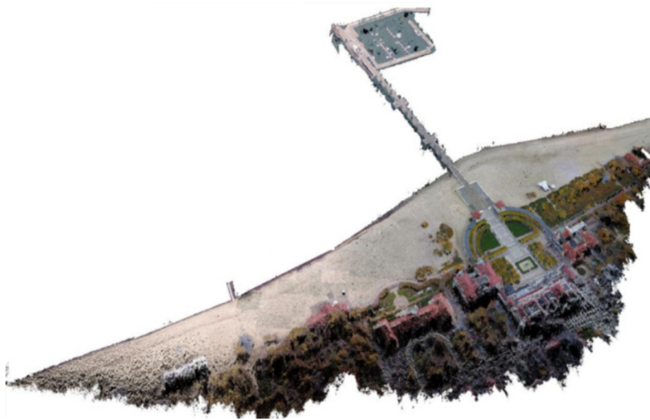
Figure 11. 3D model of the area adjacent to the Sopot pier, obtained using an unmanned aerial vehicle (UAV).
