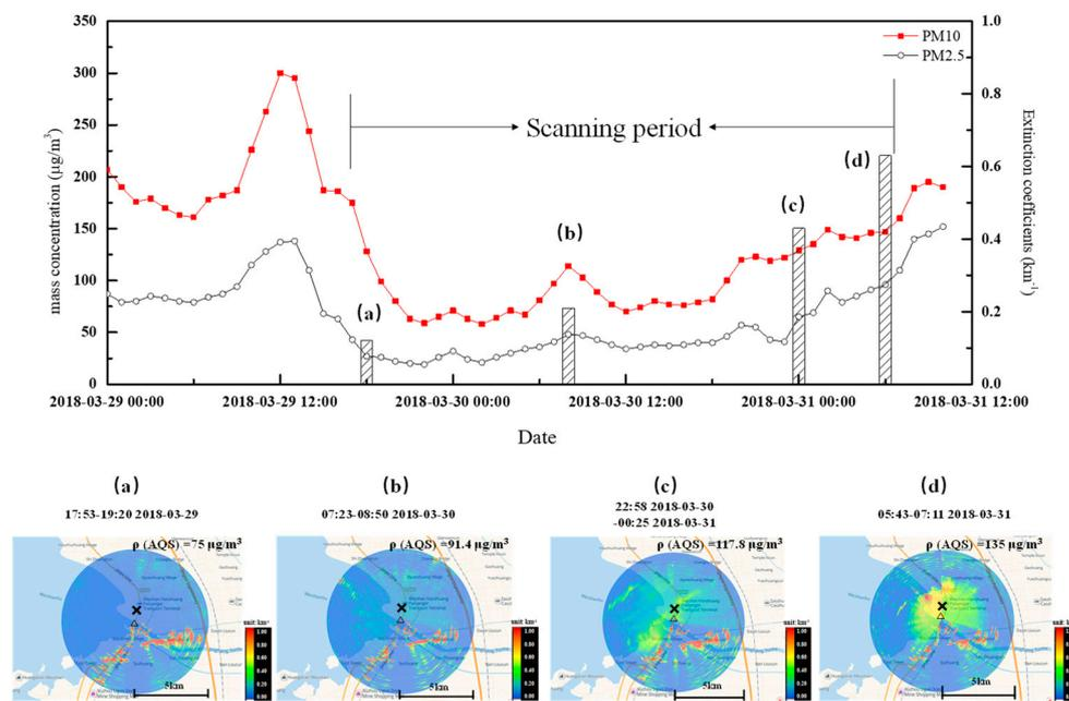
**Figure 10.** Time series of  $\rho(\text{PM}_{10})$ ,  $\rho(\text{PM}_{2.5})$  of the air quality station (AQS), and the overhead extinction coefficients of AQS from lidar (upper panel) and the aerosol mappings from lidar at Hanzhuang at 17:53–19:20, 29 March (lower pane (a)), 07:23–08:50, 30 March (lower pane (b)), 22:58, 30 March–00:25, 31 March (lower pane (c)), and 05:43–07:11, 31 March (lower pane (d)) ( $\Delta$ , the position of lidar, LS,  $\times$ , the position of AQS).
