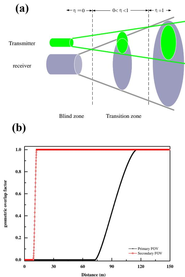
**Figure 2.** (a) The typical geometric overlap factor (GOF) of the traditional dual-axis Mie-lidar and (b) the calculated GOFs of primary and secondary FOVs. The effects of the intersection angle were ignored in the calculation of the secondary FOV.
