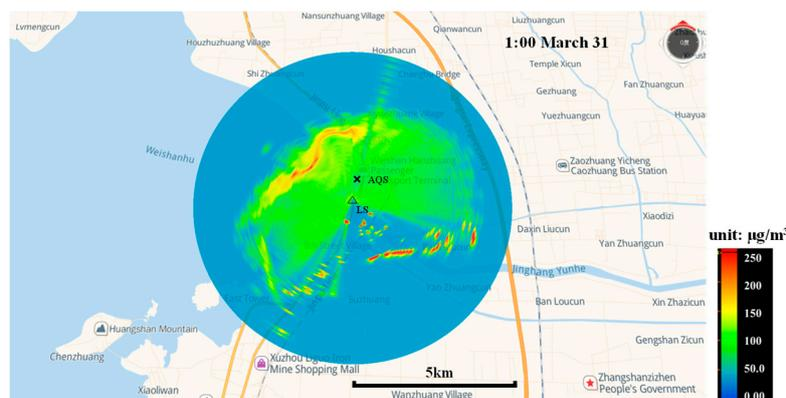
**Figure 12.** Level mass concentration distribution of aerosols at 1:00, 31 March, of dual-FOV lidar (at altitude of 22 m). ( $\Delta$ , the position of lidar, LS.  $\times$ , the position of air quality station, AQS).
