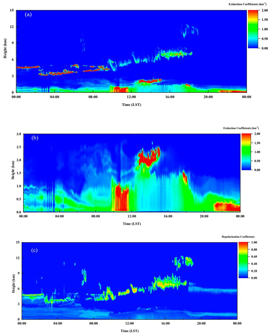
**Figure 8.** Vertical profile of aerosol detected by dual-FOV lidar. (a) Aerosol extinction coefficients in 15 km. (b) Aerosol extinction coefficients in 3 km. (c) The depolarization coefficients at 532 nm on 14 April 2019.
