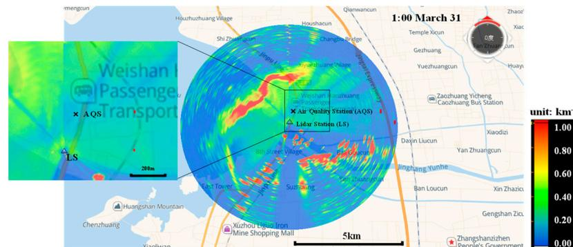
**Figure 9.** Horizontal extinction coefficient distribution of aerosols at 1:00, 31 March. Sub-chart illustrated the aerosol distribution in the region between lidar station (LS) and air quality station (AQS) on 31 March. ( $\Delta$ , the position of LS.  $\times$ , the position of AQS).
