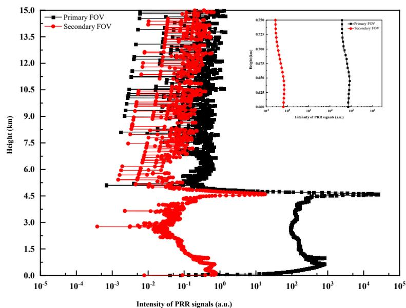
**Figure 4.** Intensities of backscattering range-corrected signals (PRR) from primary FOV (black square line) and secondary FOV (red dot line). A case of the primary (black square line) and secondary FOV PRR signal (red dot line) at the combining region of 0.6~0.75 km is shown in the sub-chart.
