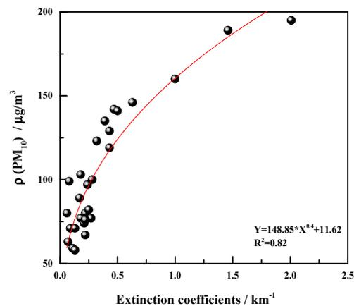
**Figure 11.** Fitting result with extinction coefficients and  $\rho(\text{PM}_{10})$ .
