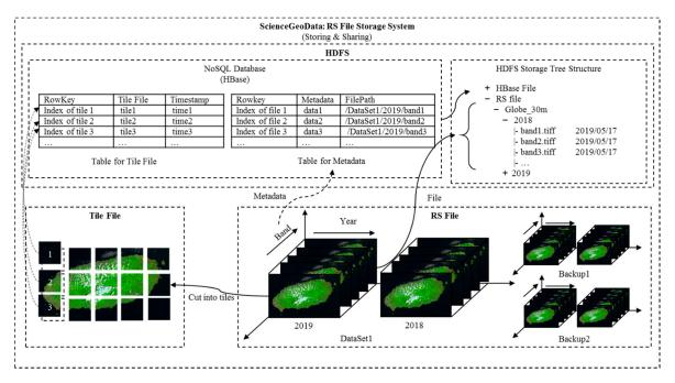
Figure 2. Remote sensing data system with a Hadoop Distributed File System (HDFS) and HBase.
