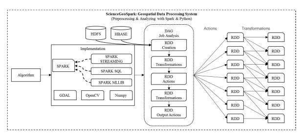
Figure 5. Programming model with Spark and Python.
