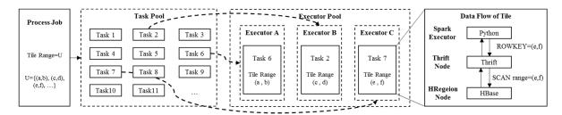
Figure 6. Data flow between HBase and Spark.
