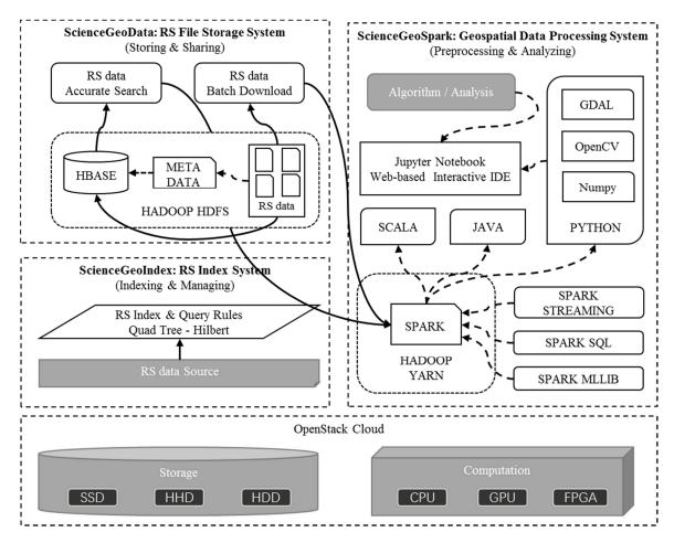
Figure 1. Architecture of ScienceEarth prototype.
