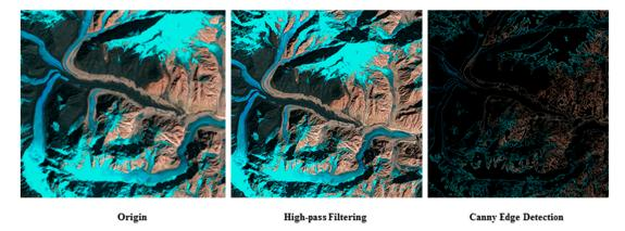
**Figure 13.** Origin, high-pass filtering, and Canny edge detection.
