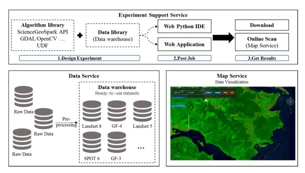
**Figure 7.** Service modules of ScienceEarth, i.e., experiment support service, data service, and map service.
