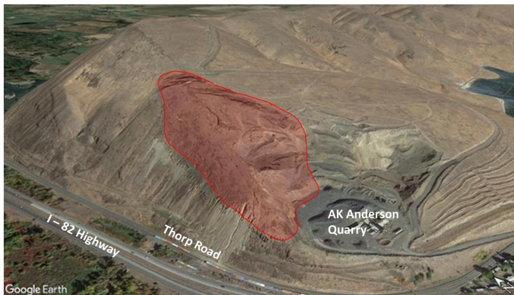
**Figure 2.** Rattlesnake Hills Landslide (red polygon), 3D view from Google Earth. The image, recorded in October 2018, reports the intense fracture field on the top of the landslide mass that moved toward the AK Anderson quarry. Some structures installed along the Thorp Road for protecting the I-82 highway from rock falls are also visible at the base of the western flank of the ridge.
