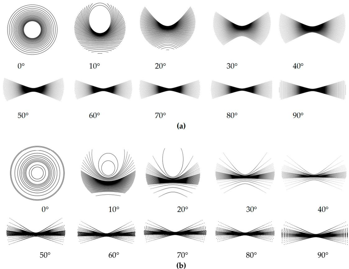
**Figure 8.** Stationary scanning patterns at a scanning range of 20 m on the ground. (a) OS-1-64. (b) Pandar64.
