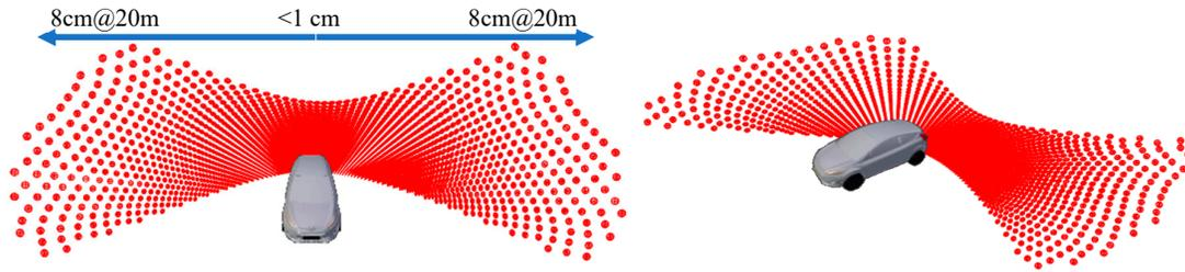
**Figure 5.** Errors representation of a scanned road surface by a single multi beam Lidar mounted at the rear part of a car roof.
