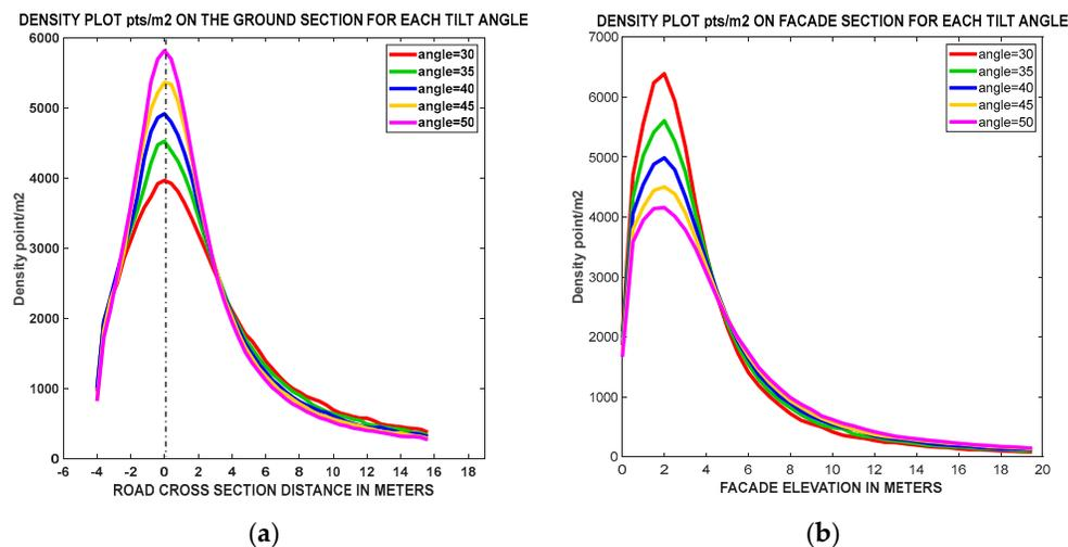
**Figure 14.** Pandar64 density checks on selected point clouds slices. **(a)** Density computed on the ground section. **(b)** Density computed on the façade section.
