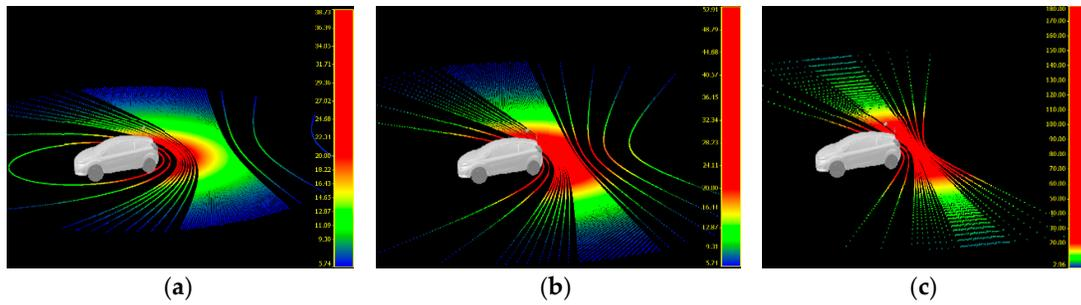
**Figure 18.** The relation between the Pandar64 Lidar tilt angle and the incidence angle where red points having  $\geq 20^\circ$  incidence angle on the ground. **(a)** @  $15^\circ$  tilting angle: the average angle of incidence  $\approx 14^\circ \pm 5^\circ$ . **(b)** @  $30^\circ$  tilting angle: the average angle of incidence  $\approx 23^\circ \pm 9^\circ$ . **(c)** @  $50^\circ$  tilting angle: the average angle of incidence  $\approx 44^\circ \pm 22^\circ$ .
