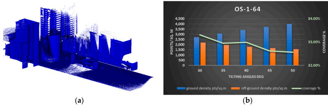
**Figure 20.** Point cloud density of OS-1-64 on the ground and off ground features and their achieved coverage percentage. **(a)** Point cloud @30°. **(b)** Graphical representation of the coverage and density achieved.
