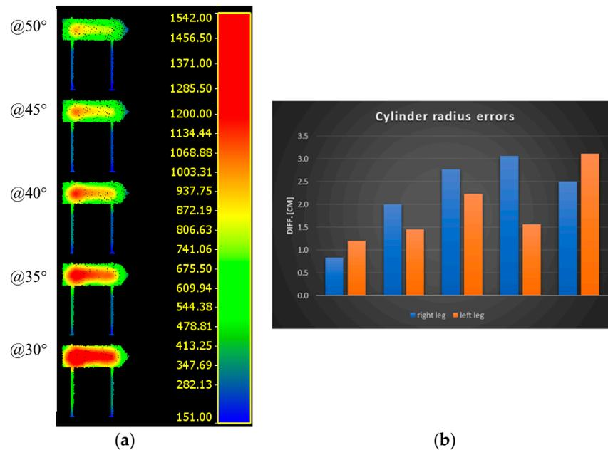
**Figure 25.** (a) Density of points at the road board sign at each tilting angle (red  $\geq 1200$  pts/m<sup>2</sup>). (b) Histogram of differences in the estimated cylindrical board legs radii.
