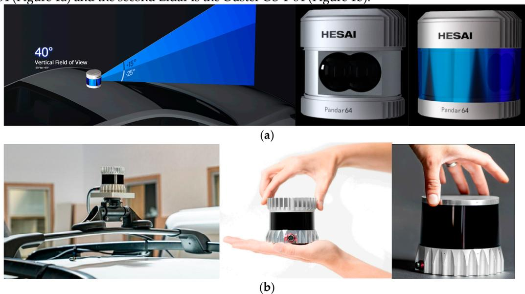
**Figure 1.** (a) Pandar64 [11]. (b) Ouster Lidar types [13,15].
