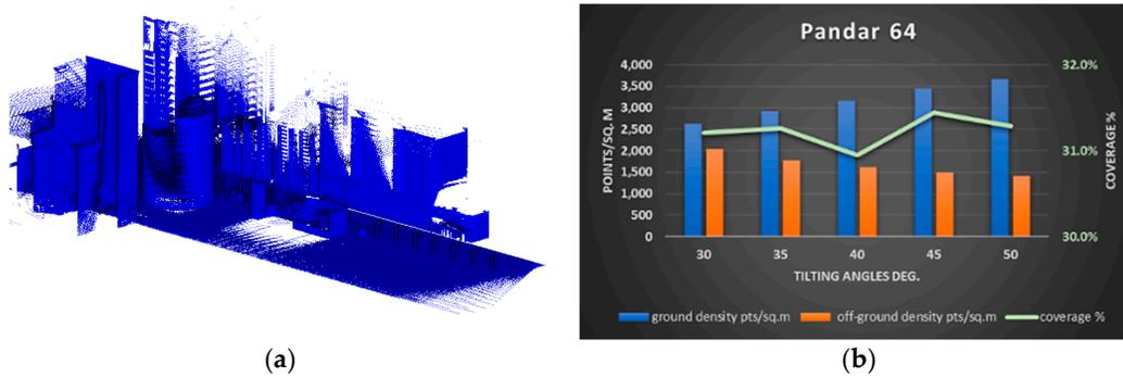
**Figure 13.** Pandar64 point cloud density on the ground and off ground features and their achieved coverage percentage. **(a)** Point cloud @30°. **(b)** Graphical representation of the coverage and density achieved.
