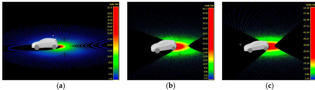
**Figure 24.** The relation between the OS-1-64 Lidar tilt angle and the incidence angle where red points having  $>20^\circ$  incidence angle on the ground. **(a)** @ 15° tilting angle: the average angle of incidence  $\approx 12^\circ \pm 8^\circ$ . **(b)** @ 30° tilting angle: the average angle of incidence  $\approx 20^\circ \pm 11^\circ$ . **(c)** @ 50° tilting angle: the average angle of incidence  $\approx 30^\circ \pm 16^\circ$ .
