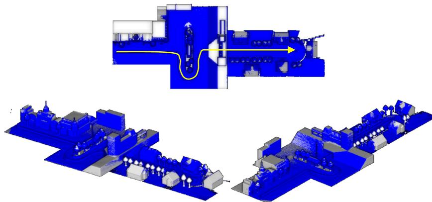
**Figure 6.** Coverage evaluation where blue color represents the scanned point cloud subtracted out of the simulated reference gray point cloud.
