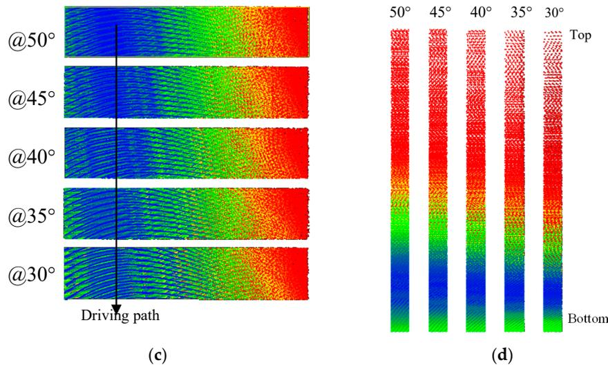
**Figure 23.** Accuracy labeled point clouds scanned by OS-1-64 (red  $\sigma \geq 5$  cm). **(a)** Accuracy at 50° Lidar tilt angle. **(b)** Accuracy at 30° Lidar tilt angle. **(c)** Accuracy estimated at the ground slice for every tilting angle. **(d)** Accuracy estimated at the façade slice for every tilting angle.
