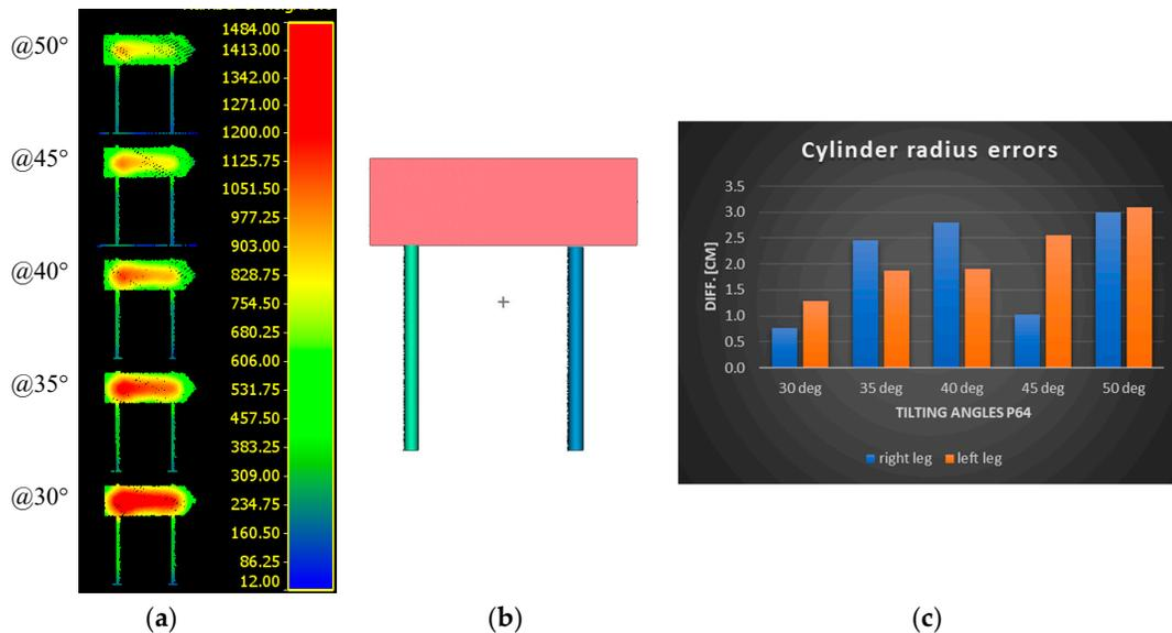
**Figure 19.** **(a)** Density of points at the road board sign at each tilting angle (red  $\geq 1200$  pts/m<sup>2</sup>). **(b)** An example of the detected primitives of the board sign. **(c)** Histogram of differences in the estimated cylindrical board legs radii.
