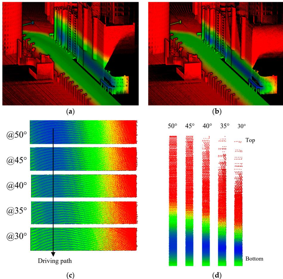
**Figure 17.** Accuracy labeled point clouds scanned by Pandar64 (red  $\sigma \geq 5$  cm) (a) Accuracy at 50° Lidar tilt angle. (b) Accuracy at 30° Lidar tilt angle. (c) Accuracy estimated at the ground slice for every tilting angle. (d) Accuracy estimated at the façade slice for every tilting angle.
