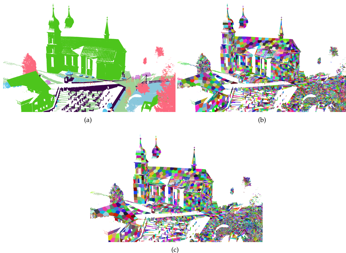
Figure 7. The 10,000 supervoxels generated by our merge-swap method with and without adaptive octree-based merging, respectively, from 5.5 million input points. (a) The ground truth; (b) result with octree-based merging and BR = 0.7002 , UE = 0.1471 , GCE = 0.0132 , and running time = 80 s; and (c) result without octree-based merging and BR = 0.6975 , UE = 0.1434 , GCE = 0.0137 , and running time = 4.5 min.
