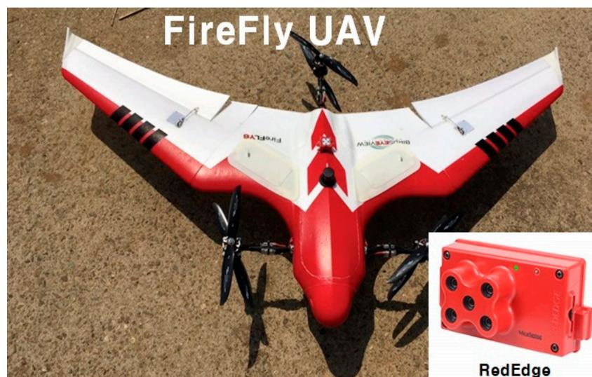
Figure 2. Firefly UAV and RedEdge multispectral camera.
