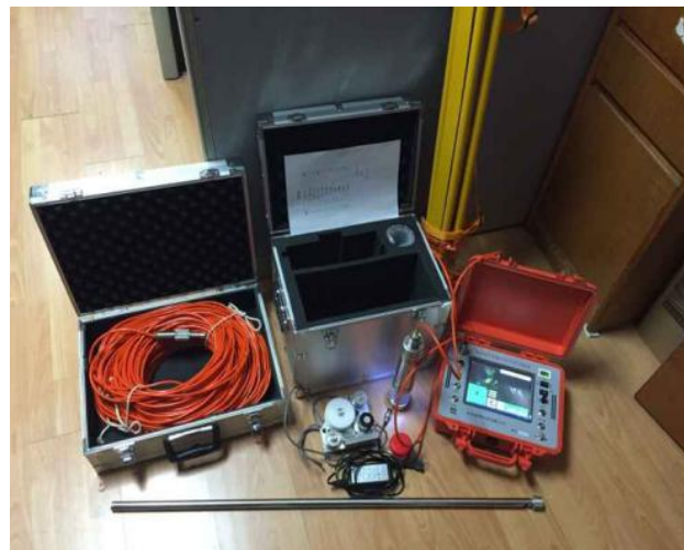
Figure 11. The GD3Q-GA panoramic borehole televiewer.
