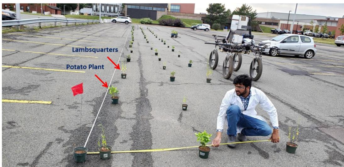
**Figure 6.** Design of the laboratory experiment for testing of smart variable rate sprayer. The experimental setup consisted of 60 m long and 2.74 m wide strips of randomly arranged healthy, simulated diseased, and weed plants.
