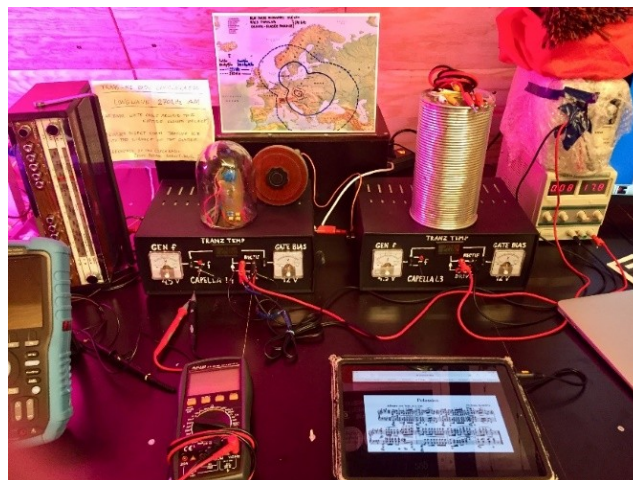
Figure 12. Both IGLUNA 2019 longwave transmitters inside the simulated lunar habitat in the Glacier Paradise, 3868 m a. s. l. The modulation (acoustic) signal is generated directly by a tablet for the ‘glass dome’ transmitter and by an STM32-based microcontroller circuit for the ‘Thermos’ transmitter. The Jowita 2 radio receiver for on-site modulation control can be seen on the left. The pink glow of the stand is created by one of the nearby experiments. The map above the transmitters shows the signal coverage of 225 kHz (Solec Kujawski) and 270 kHz (Topolná) for comparison. Photograph by the Author.
