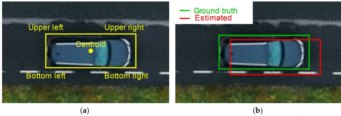
Figure 4. (a) Characteristic points of bounding boxes; (b) example of difference between ground truth and estimated bounding boxes.
