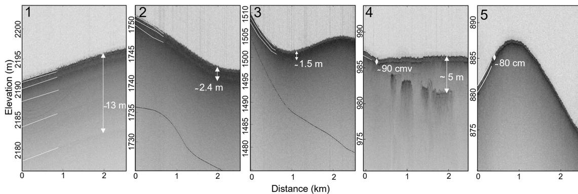
**Figure S4.** Stratigraphy of the upper layers as seen by the UWB-M radar in 2018. In the accumulation zone the stratigraphy can be resolved down to 13 m, with a decline to 1.5 m at the onset of the ablation zone (Panel 1-3). Panel (4) displays the cross section over a supraglacial lake with a frozen surface and a snow layer on the lake ice. Panel (5) displays the layer of the last summer prior to the impurity covered area. Further downstream no reflections of the last summer were found at all.
