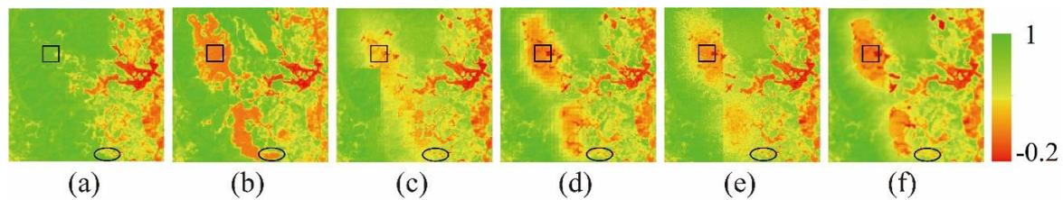
**Figure 14.** Visual comparison of inset map in urban area. (a,b). Original Landsat\_NDVI inset map 1 November 2000 and 7 November 2002; (c–f). Predicted Landsat\_NDVI inset map by ESTARFM, NDVI-LMGM, FSDAF, and NDVI\_FMHC.
