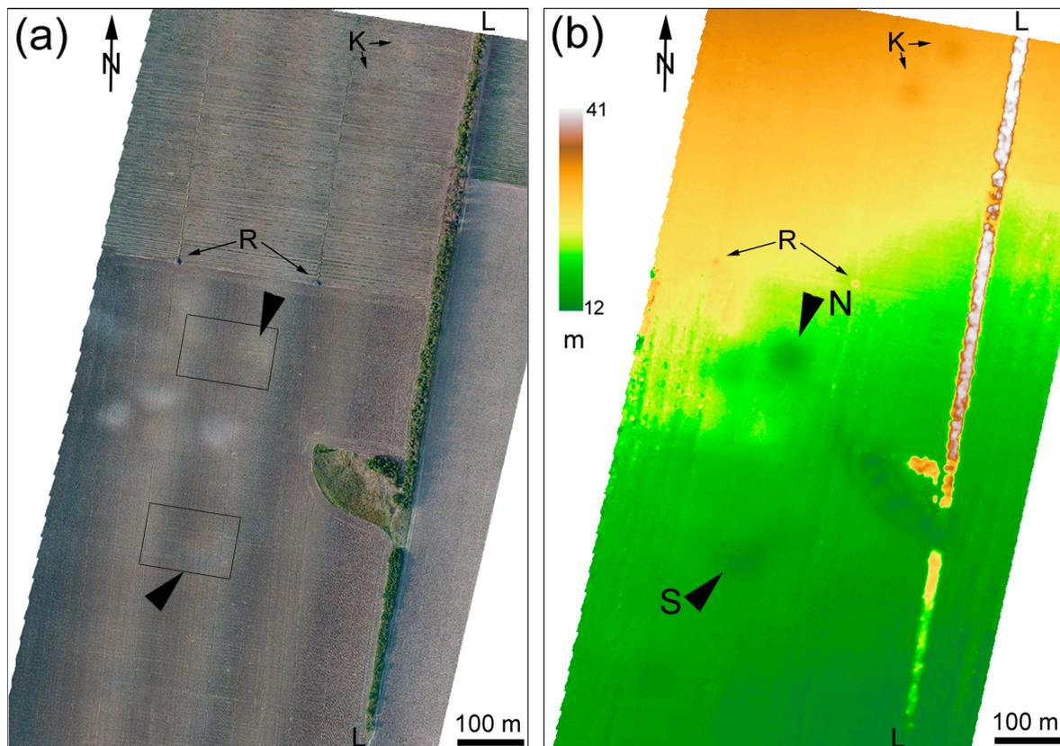
**Figure 6.** The study site: (a) UAS-based orthomosaic. Two black frames show the position of two images displayed in Figure 4c,d. (b) Elevation map. Two big arrows show the Northern (N) and Southern (S) ring microstructures detected by the geomorphometric analysis (see Figures 7 and 8). LL—a windbreak; R—mounds of agricultural refuse; K—probably, kurgans. For the position of the study site, see Figure 5a, the yellow frame.
