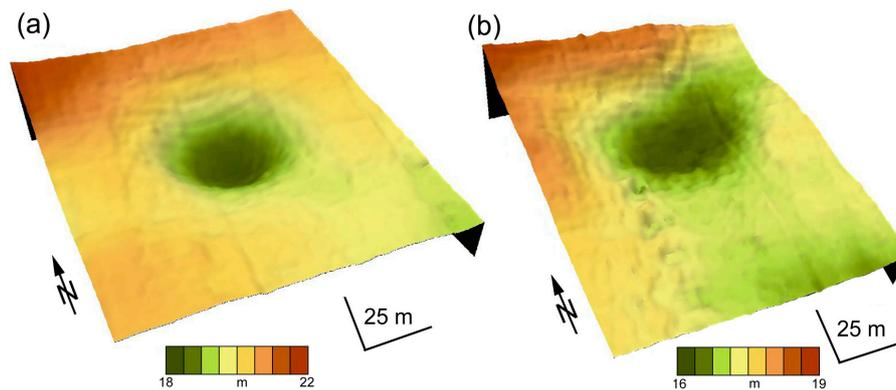
**Figure 8.** Three-dimensional models of the two ring microstructures detected by the geomorphometric analysis: (a) the Northern microstructure, (b) the Southern microstructure.  $20\times$  vertical scale exaggeration is used. For the microstructure locations, see Figure 6b.
