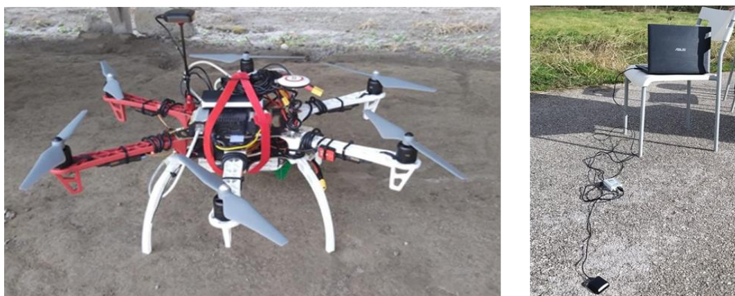
Figure 1. Multicopter-UAVs (M-UAV) radar imaging system: (left) M-UAV hexacopter with onboard equipment [21]; (right) ground-based Global Positioning System (GPS) station [21].
