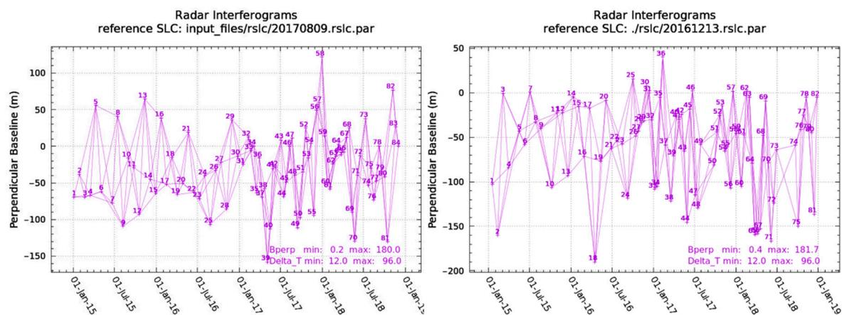
Figure 3. Baseline vs. time plots (left) ascending orbit data (right) descending orbit data.
