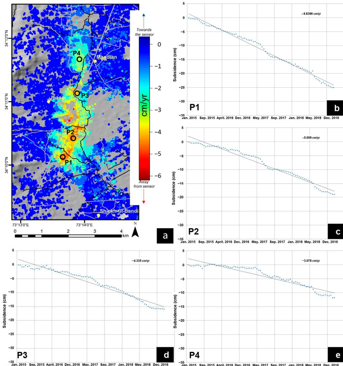
**Figure 8.** Time series evaluation of averaged LOS deformation presented using ascending data: (a) location of PSs, (b) P1, (c) P2, (d) P3, and (e) P4.
