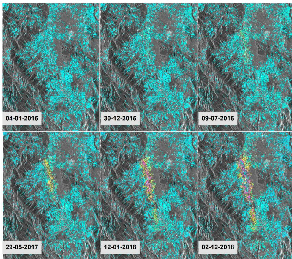
**Figure 7.** Six different stages of cumulative land subsidence pattern in RADAR geometry. The background image is the averaged intensity image of the study area. One color cycle corresponds to 10 cm/year displacement.
