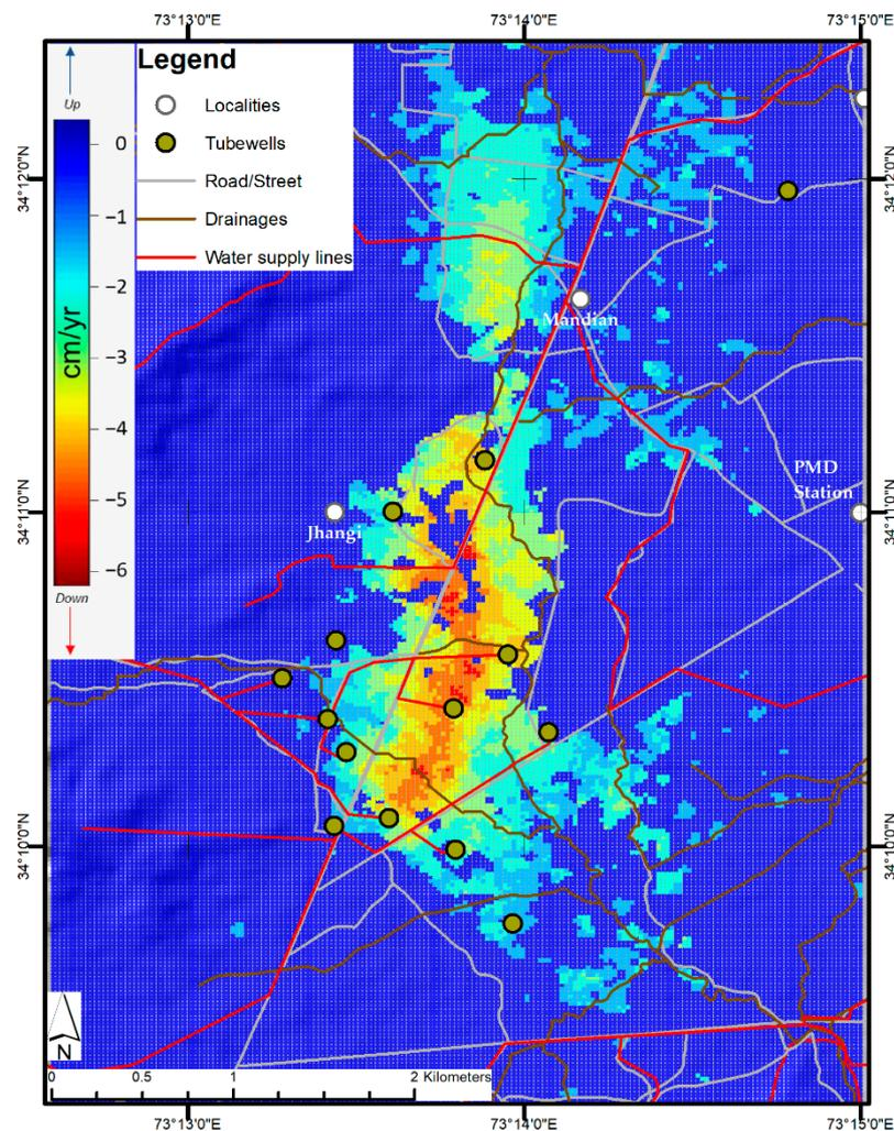
**Figure 11.** Location of tubewells and supply lines overlaid on average vertical velocity map.
