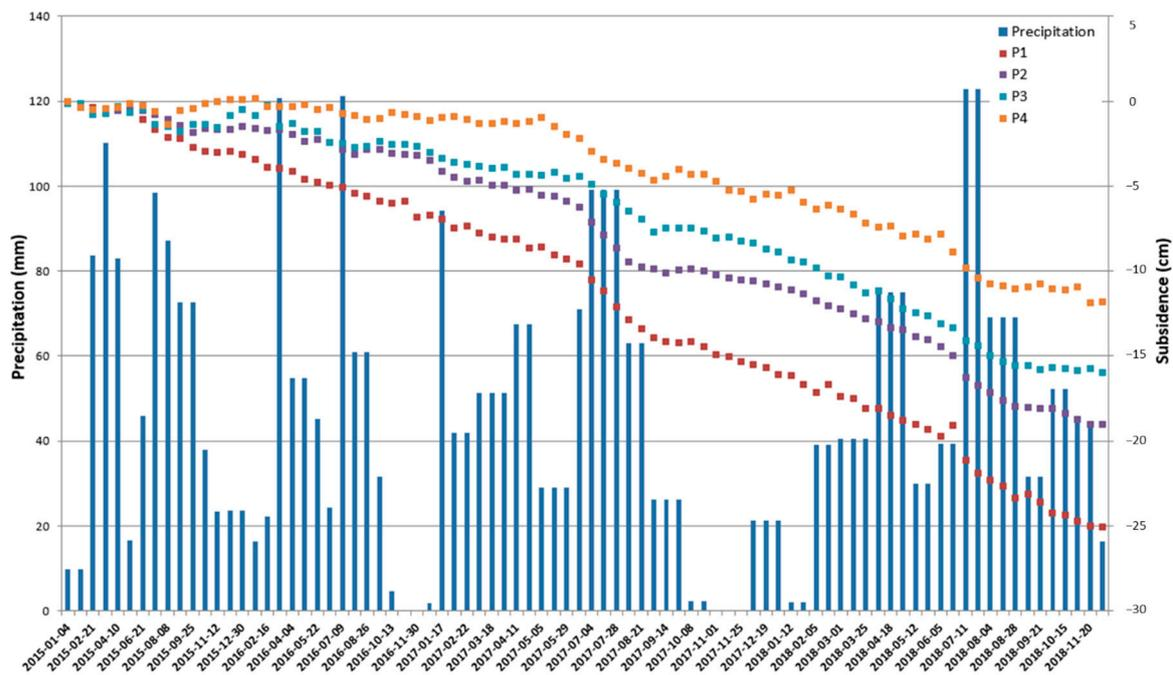
**Figure 12.** Time series LOS subsidence of PS points P1, P2, P3, and P4 versus daily precipitation at Kakul Station.
