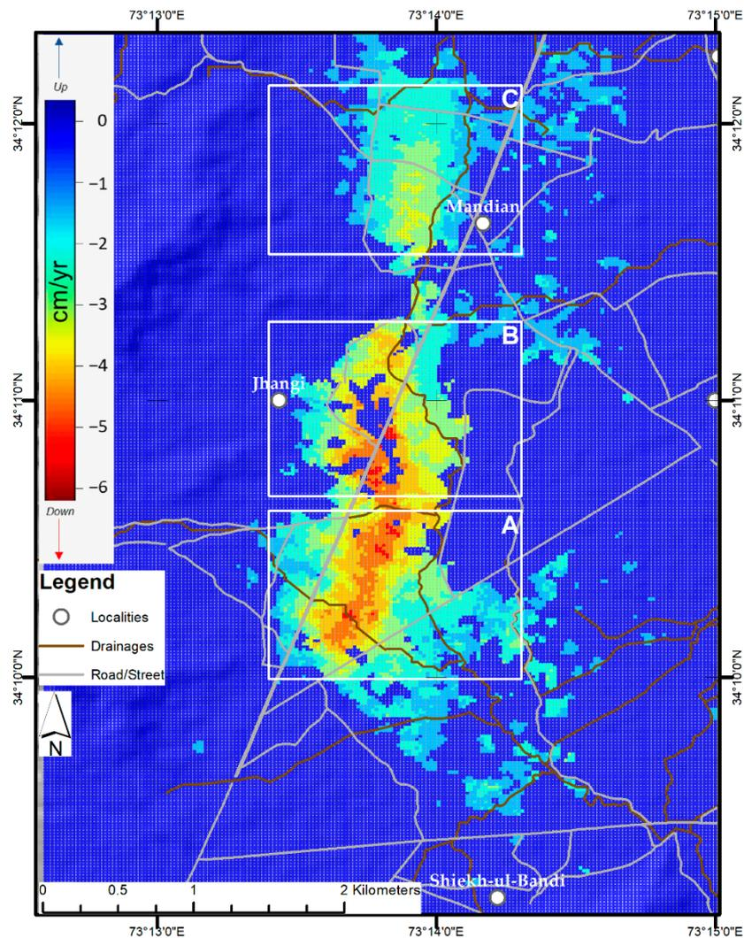
**Figure 6.** Mean vertical velocity map in cm/year. The red color represents downward movement (i.e., subsidence).
