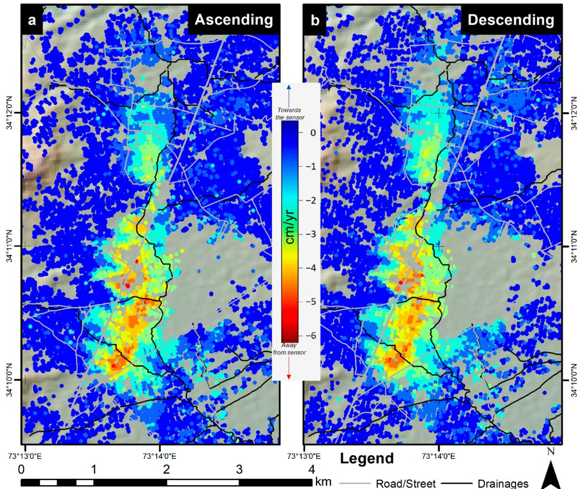
**Figure 5.** Average line of sight (LOS) velocity maps: (a) ascending and (b) descending orbits’ data.
