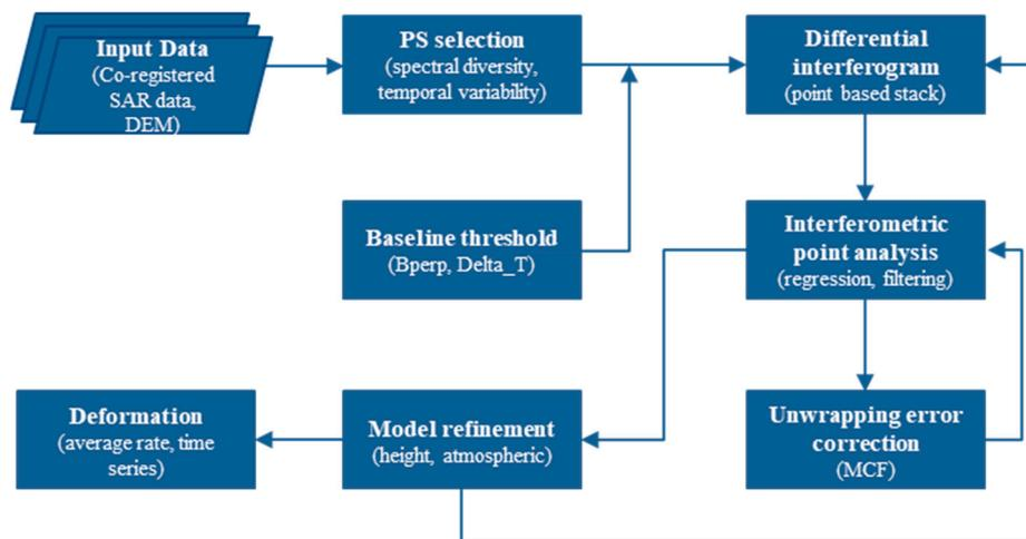
Figure 2. Processing workflow for interferometric point target analysis (IPTA).
