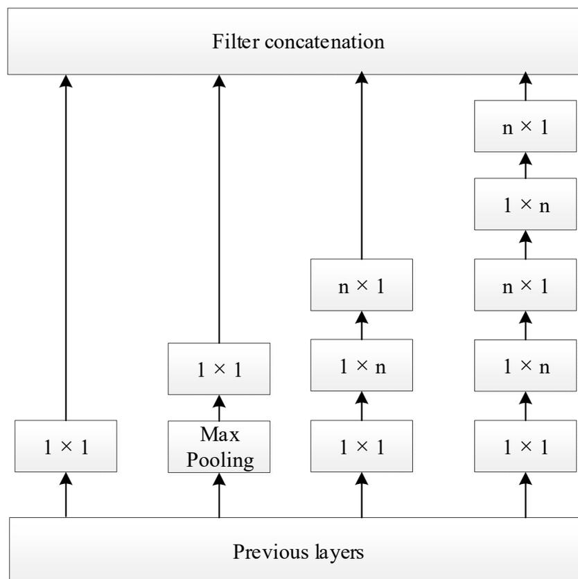
Figure 1. Inception Module structure in Inception V3.
