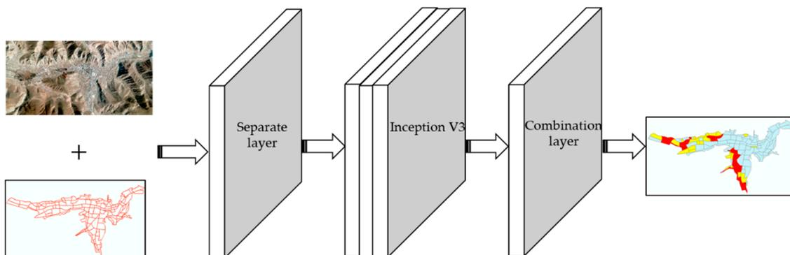
**Figure 3.** Improved CNN classification framework for damaged groups of buildings after earthquakes.
