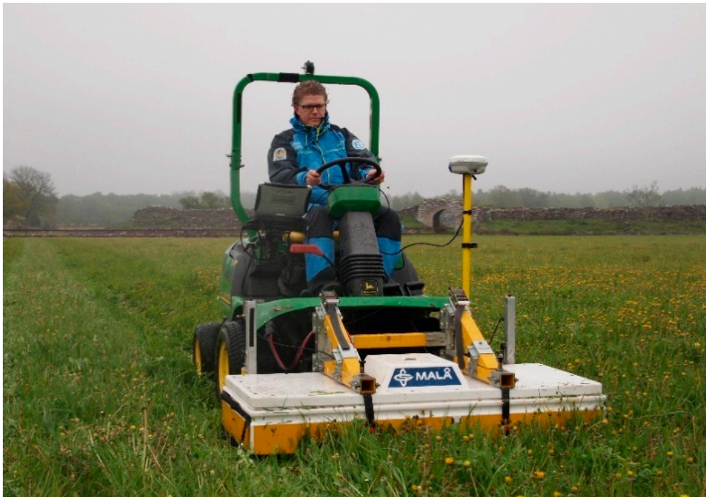
Figure 5. The 16 channel 400 MHz MALÅ Imaging Radar Array (MIRA) measuring outside Gråborg ringfort, Öland. Photo: M. Larsson (2014).
