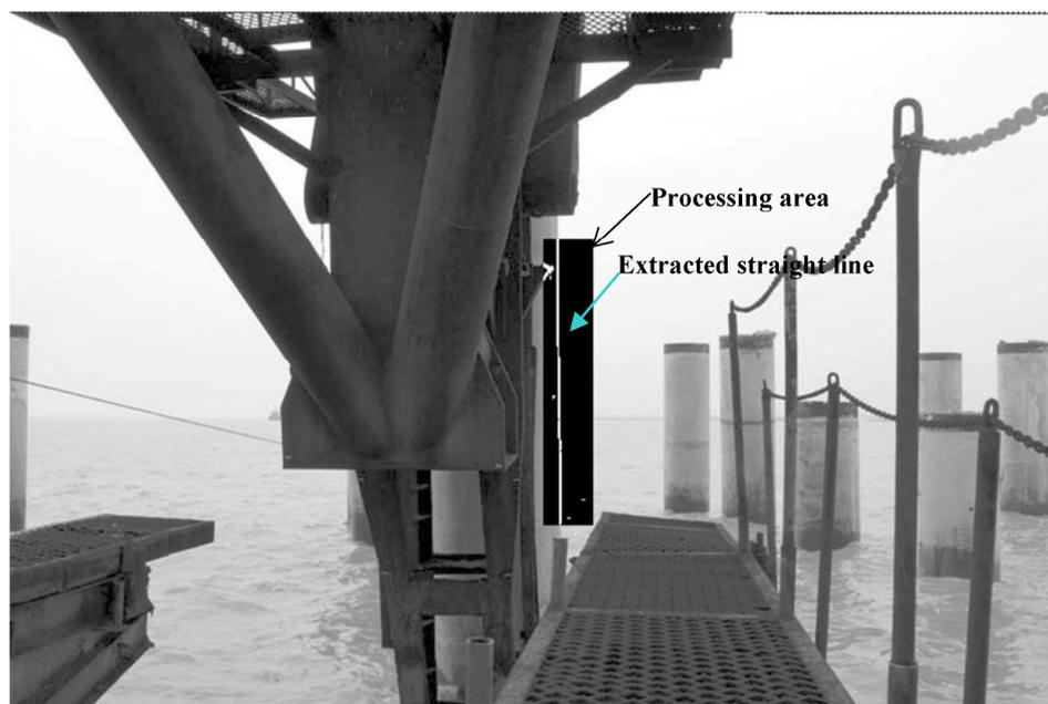
**Figure 9.** Image from the camera and extraction of the straight line of the pile edge.
