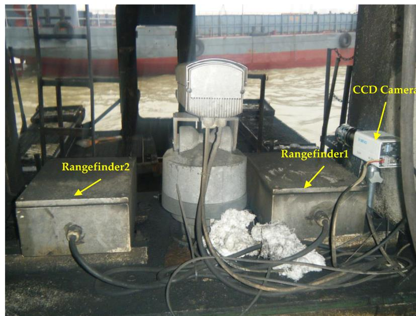
Figure 14. Rangefinders and CCD camera installed on the ship's deck.
