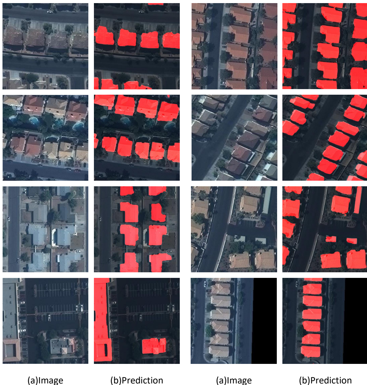
Figure 9. Examples of segmentation results of our method on mapping challenge dataset. (a) Image. (b) Prediction.
