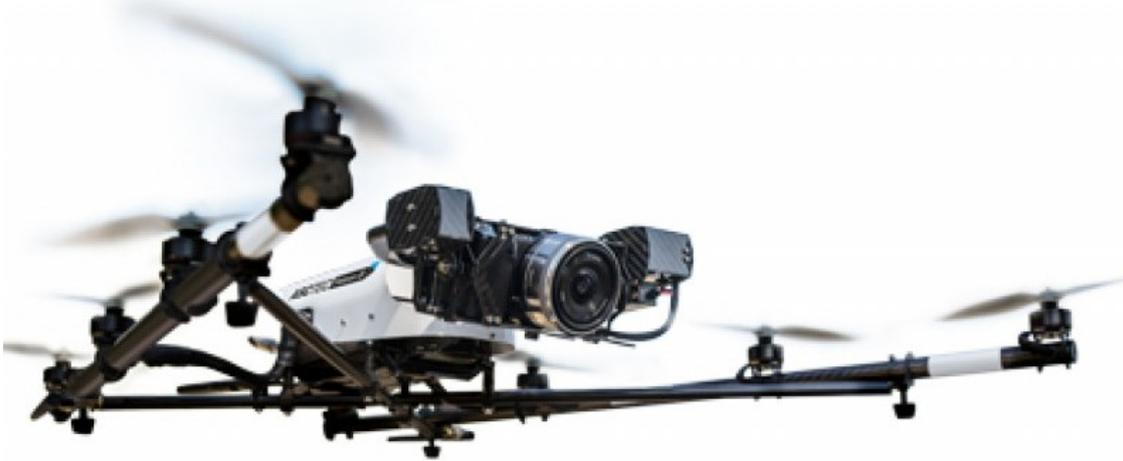
Figure 3. AscTec Falcon 8 unmanned aerial system (UAS) equipped with a SONY NEX-5 camera.
