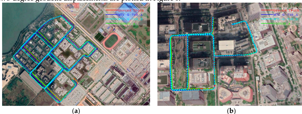
Figure 6. The trajectories with two-degree geodetic displacement of MTI-G-710 under Setting A and Setting D, and POS620 under Setting A: (a) The trajectories for the sequence WRIC, and (b) the trajectories for the sequence GFH.
