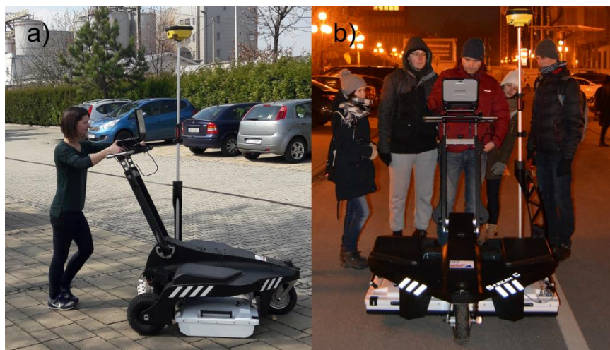
Figure 2. Ground Penetrating Radar (GPR) Leica Stream C: (a) during test measurement; (b) in urban area.
