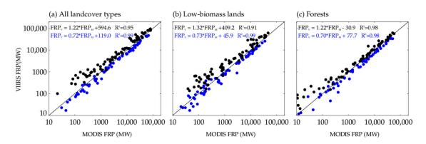
**Figure 10.** Scatter plots of the monthly total FRP of VIIRS versus MODIS. (**a**) all land cover types, (**b**) low-biomass lands, (**c**) forests. Black dots are the monthly total FRP summed from all detected fires in fire products; blue dots are the monthly total FRP summed from concurrently detected fires.
