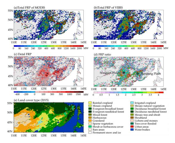
**Figure 7.** Spatial distribution of total FRP over 2012–2017 in Northeast Asia at 0.25° resolution: (a) MODIS; (b) VIIRS; (c) Delta FRP (VIIRS minus MODIS); (d) VIIRS-to-MODIS FRP ratio; (e) land cover type shown in 2015.
