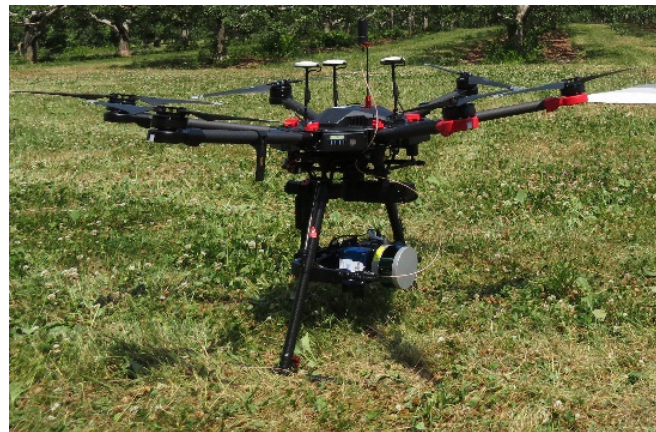
Figure 3. Image of DJI Matrice 600 Pro with Velodyne Puck mounted and pointed at nadir.
