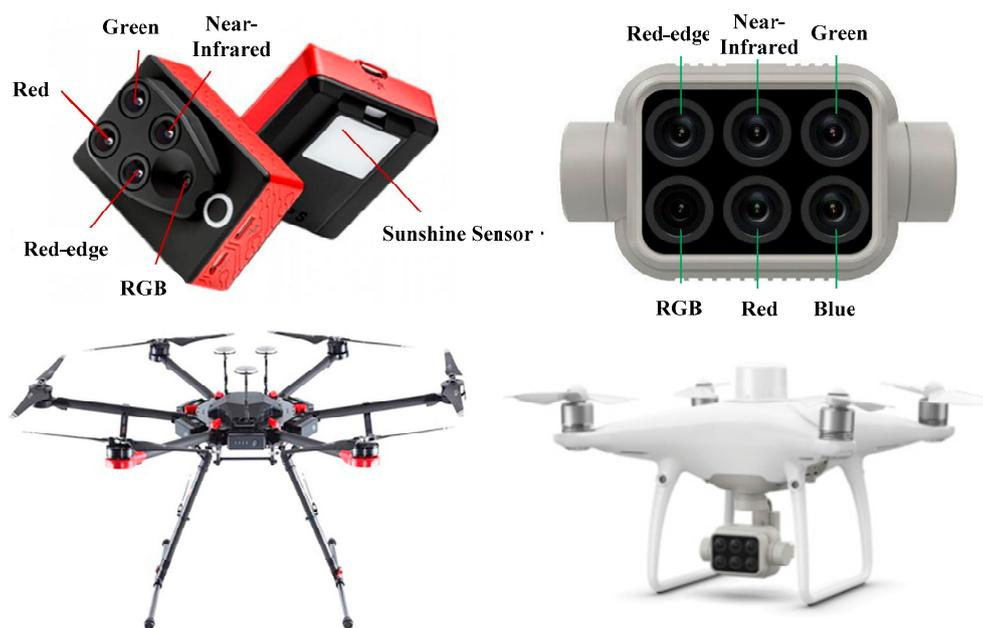
**Figure 2.** UAV platforms and multispectral sensors (Sequoia and P4M). The Sequoia sensor is carried on the EM6-800 hexacopter UAV (left), and the P4M uses its own aircraft (right).
