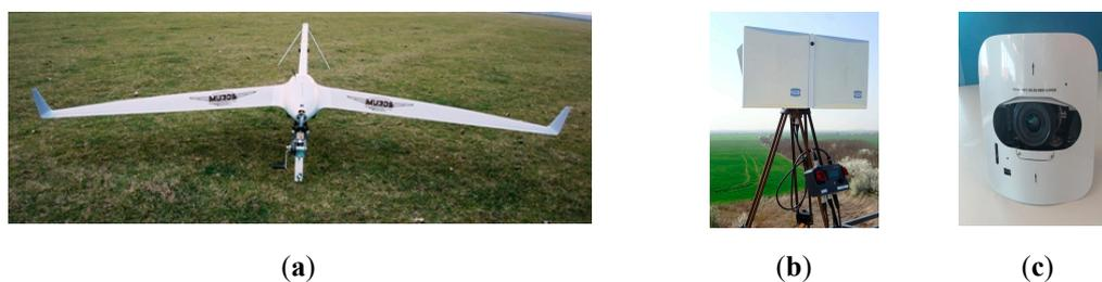
**Figure 1.** System components: (a) UAV fixed wing; (b) ground terminal, and (c) payload photo.
