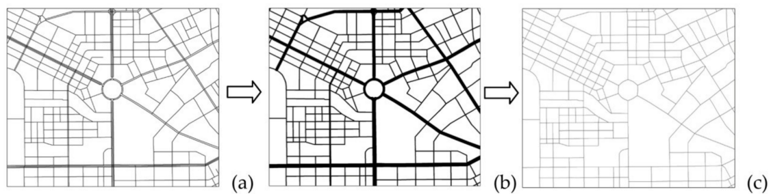
Figure 2. OpenStreetMap (OSM) data processing flow diagram. (a) Filtered OSM; (b) buffer zones; (c) centerlines.
