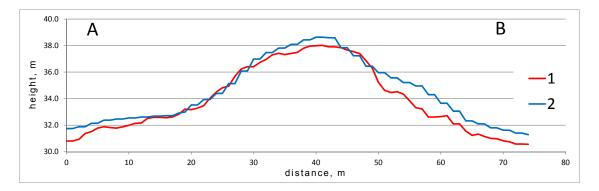
**Figure 8.** A comparison of elevation profiles plotted using the author's DSM for GEC-1 (1), with ArcticDEM (2). Both lines are not smoothened. Figure 2a shows the spatial position of the profile AB across the GEC-1 mound-predecessor.
