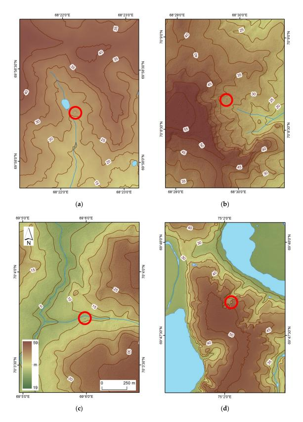
**Figure 2.** Differences in the geomorphic setting of gas emission craters identified through DSM analysis. Key site DSM fragments: (a) GEC-1, (b) GEC-2, (c) GEC-3, (d) AntGEC. Red circles indicate GEC location.
