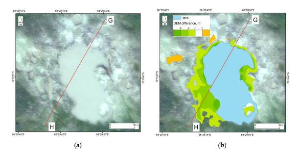
**Figure 6.** The difference between DSMs obtained "before" (2010–2011) and "after" (2013) GEC-2 formation): (**a**) WorldView-2 image dated 21 July 2013; (**b**) A fragment of DSM difference. Differences in elevation predominantly occur in a well-defined area, located southwest of the lake. See the GH profile in Figure 5.
