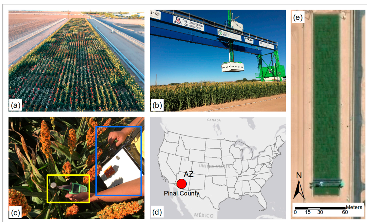
Figure 1. Location of test site and data collection. (a) Experimental field; (b) the field scanner operating in the field; (c) in-situ data collection of leaf chlorophyll concentration (LCC) using Dualex 4 Scientific (yellow box) and spectral data using PSR-3500 spectroradiometer (blue box); (d) location of study area in Pinal County, AZ; (e) a top view image of the field collected from ArcGIS Online.
