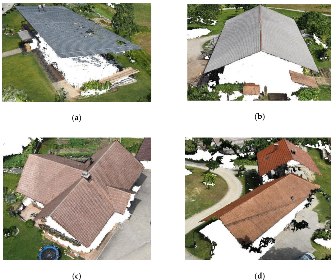
Figure 1. Selected building roof types for 3D building modelling shown in the photogrammetric point cloud: (a) flat roof; (b) gable roof; (c) cross gable roof; (d) two-level gable roof.
