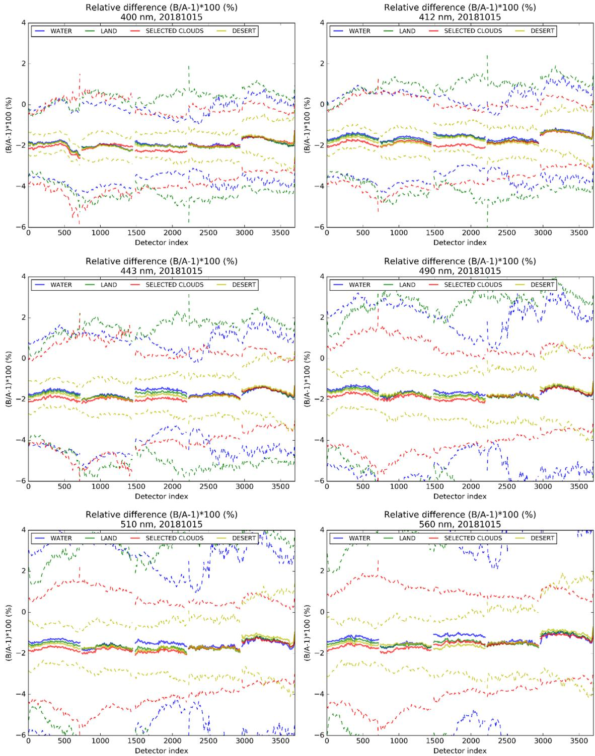
**Figure S1.** Relative differences between OLCI-A and OLCI-B homogenised reflectance per bin of instrument detectors for water (blue), land (green), selected clouds (red), and desert (yellow). Bands Oa01 (400 nm), to Oa06 (560 nm). Dashed lines indicate the standard deviation. Tandem data from October 15<sup>th</sup>, 2018.
