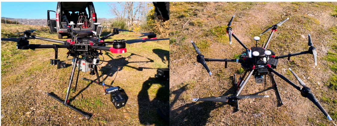
**Figure 2.** Aerial Light Detection and Ranging (LiDAR) system used for the survey.
