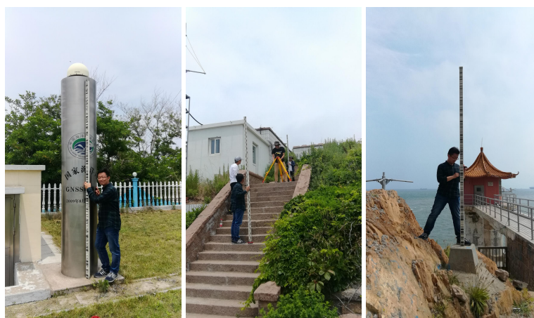
Figure 6. The spirit leveling work between the GNSS permanent station and the tide gauge at station XMD. The left-hand photo is of the permanent GNSS station; the middle photo shows the leveling work between the GNSS and the benchmark of the tide gauge; and the right-hand photo shows the benchmark of the tide gauge and the tide station.
