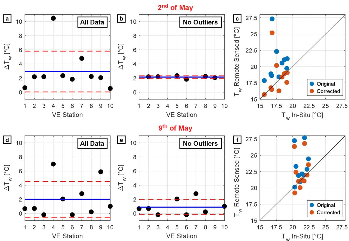
**Figure 3.** Correction of retrieved water temperature for May the 2nd (a–c) and for May the 9th (d–f). (a,d) and (b,e) show the temperature differences between retrievals from satellite data and measurements collected by the probes with all data and after the deletion of the outliers, respectively. The blue line highlights the mean difference, whereas the red dotted lines highlight the standard deviation. Original and corrected temperature data are summarized in (c,f).
