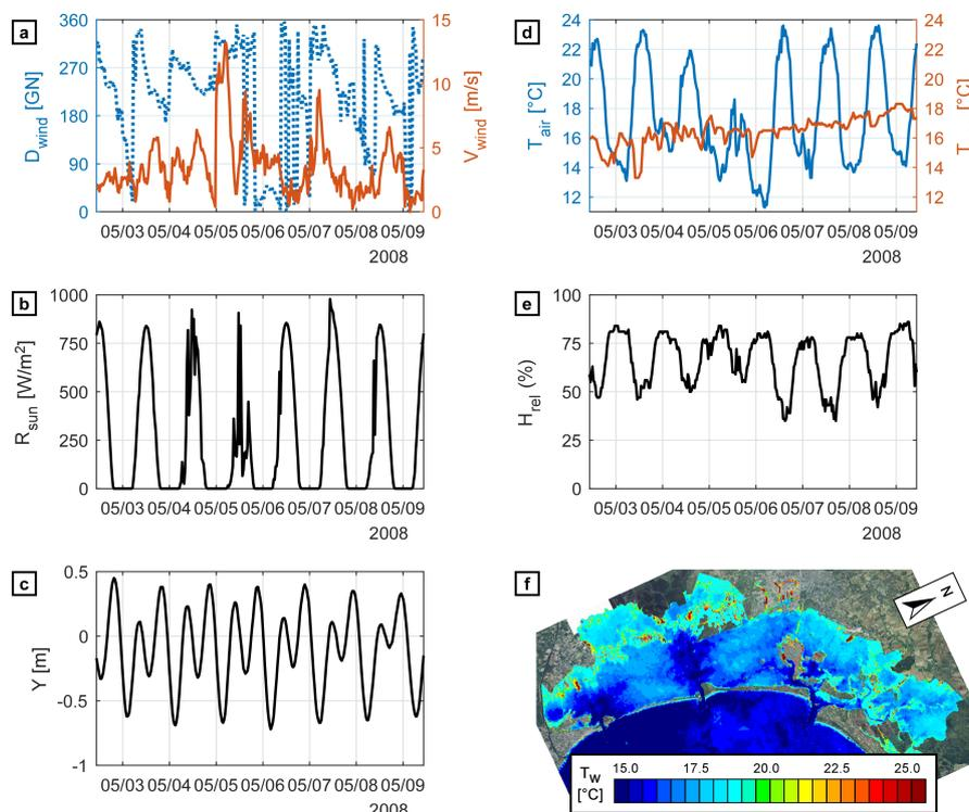
**Figure 2.** Time series of (a) wind direction,  $D_{wind}$ , and speed,  $V_{wind}$ ; (b) solar radiation measured at the surface,  $R_{sun}$ ; (c) water level,  $Y$ ; (d) air temperature,  $T_{air}$ , and sea water temperature,  $T_{sea}$ ; (e) relative humidity,  $H_{rel}$ , used as boundary conditions. (f) Remote sensed water temperature spatial distribution used as initial condition.
