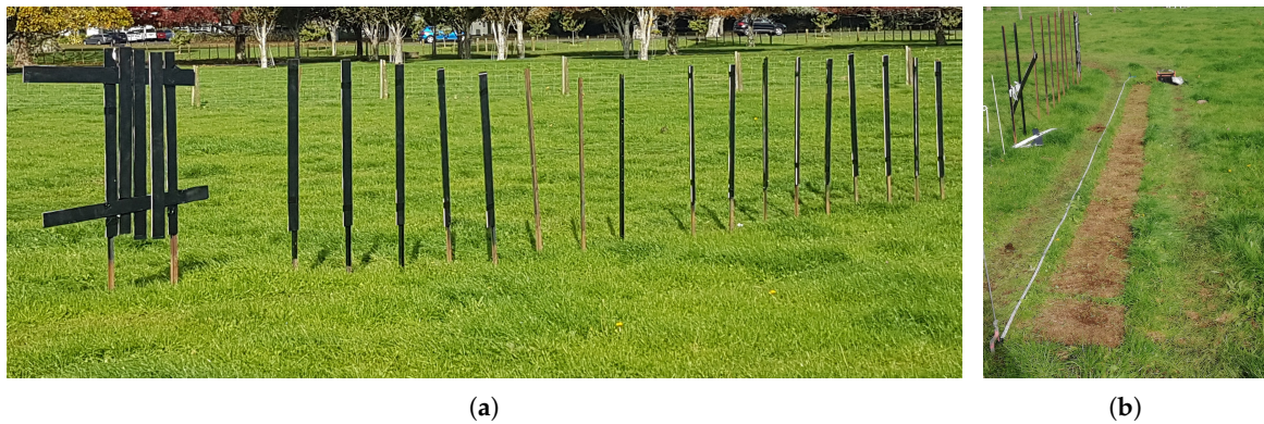
Figure 20. Photo (a) shows “Transect 2” which was used for bike field trials. The black cards on posts were used for localisation of ultrasonic measurements using the IR sensor. Photo (b) shows the same transect with the grass cut to the ground for cut, dry and weigh biomass measurements.
