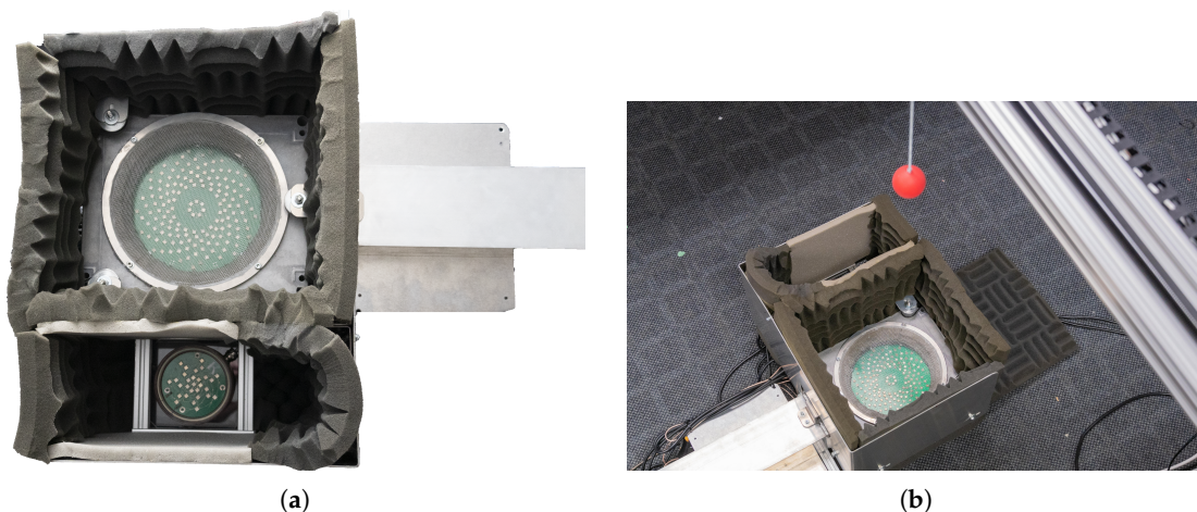
Figure 16. Photo (a) shows the V1 and V2 arrays mounting for farm bike trials. Photo (b) shows the experimental setup used for beam pattern measurements.
