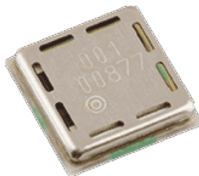
Figure 4. Murata MA40H1S-R surface mount transducer.
