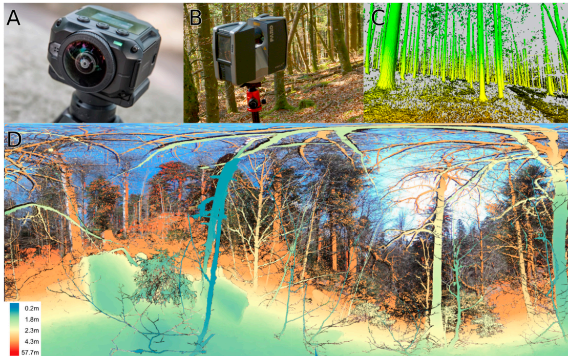
Figure 3. (A): Garmin VIRB 360 digital camera; (B) Faro Focus 120 terrestrial laser scanner; (C): Visualization of a point cloud; 2D: overlay of the 360°-image from the camera with the distance image from the scanner - blue colors indicate closer red colors more distant points.
