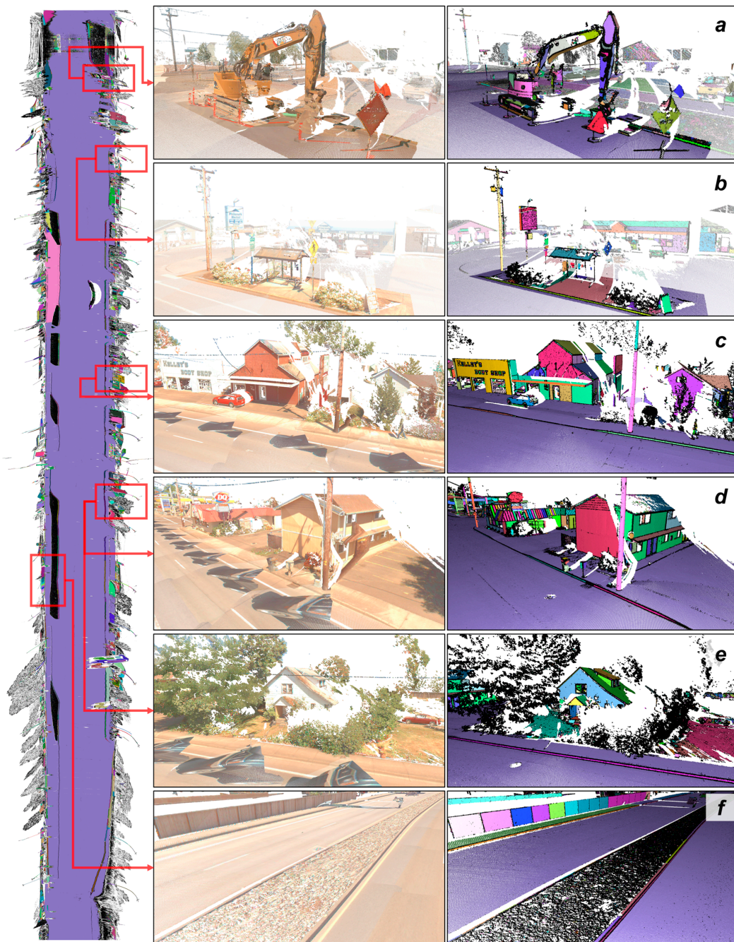
Figure 10. Overview of the segmentation result in a scan pattern grid (left) and close-up views to the point cloud of the segmentation results on various objects: (a) an excavator; (b) a bus station; (c–e) different types of buildings; (f) fences and median filled with rocks.
