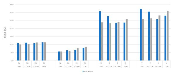
**Figure 3.** Root-mean-square errors (RMSEs) of the stand level (n = 150) predictions for D<sub>g</sub>, H<sub>g</sub>, G, and V. Predictions were made using two different single-tree positioning methods for deriving forest inventory attributes for sample plots (XY<sub>H</sub>, XY<sub>HH</sub>) and with four different sample plot sizes. Note that sample plot size is given as the radius (in m) of the sample plot, not the area (in m<sup>2</sup>). See also data from Table 2.
