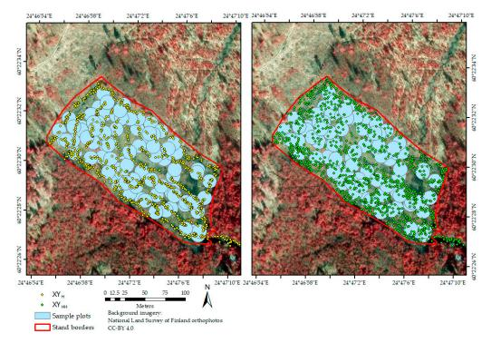
**Figure 2.** One of the modeling stands in the study area, showing 100 generated sample plots (r = 9 m). Left: the location of each tree is determined based on the harvester's GNSS position (XY<sub>H</sub>). Right: the location of each tree is based on the computationally derived harvester head position (XY<sub>HH</sub>).
