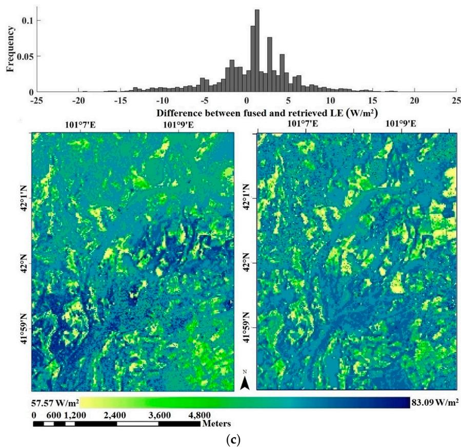
**Figure 4.** Histogram (top panel) of the difference between fine-resolution LE data fused by the SADFAET (right panel) and the estimates directly retrieved by the ESVEP model using Landsat 8 data (left panel) on (a) May 15, (b) July 18 and (c) August 28.
