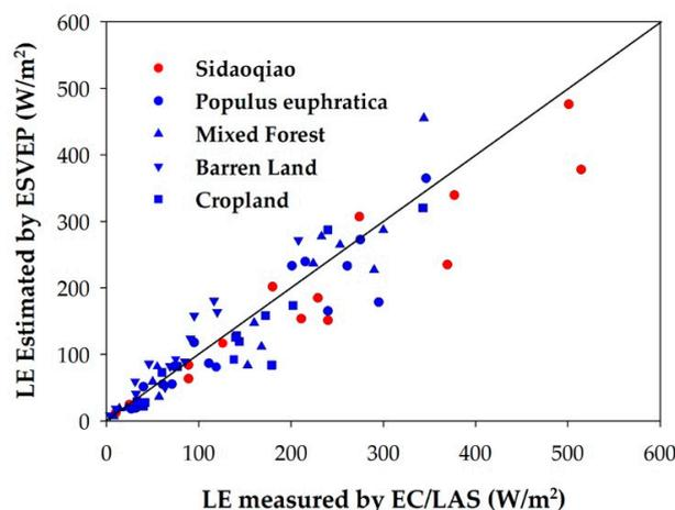
**Figure 3.** Validation of the instantaneous LE estimations from the end-member-based soil and vegetation energy partitioning (ESVEP) model for MODIS- and Landsat-based retrievals against ground-based LAS (red symbols) and EC (blue symbols) measurements.
