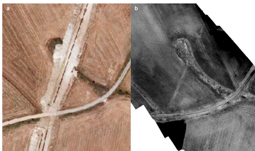
Figure 3. (a) The NDVI positive anomaly created by the service trench. (b) The 2005 service trench seen in the geoEuskadi aerial photograph [60].
