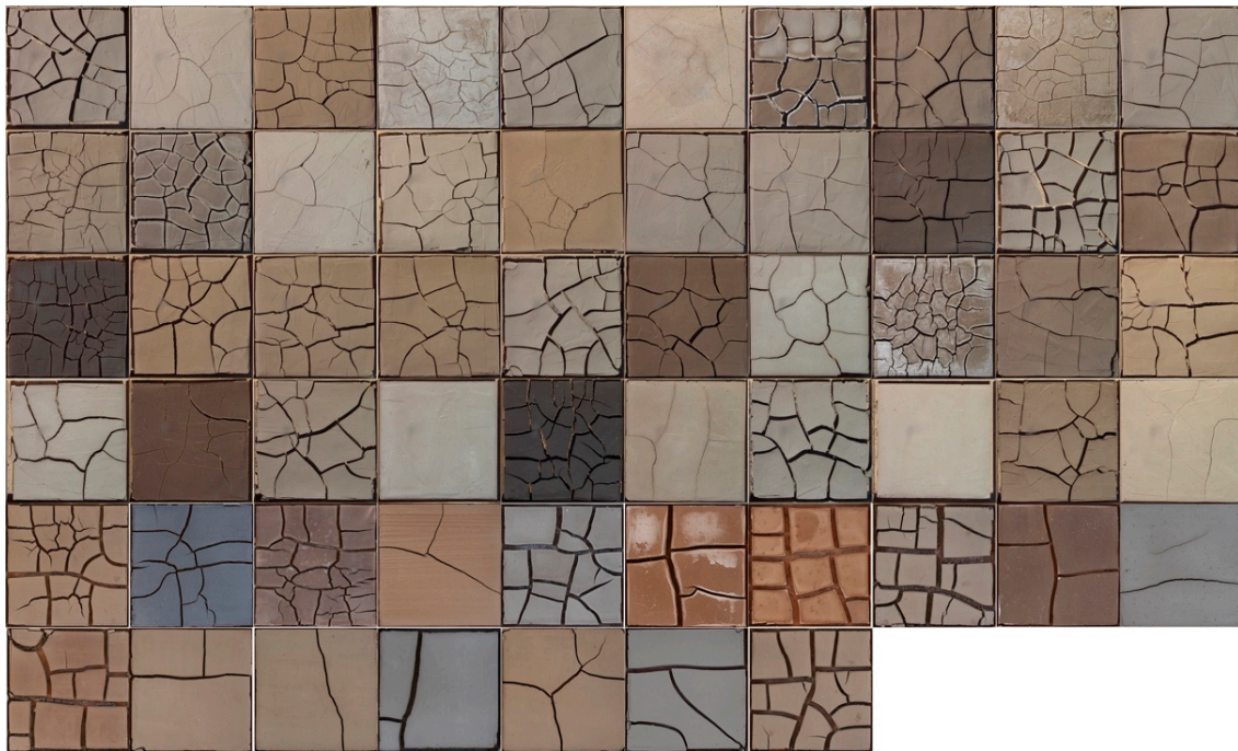
Figure 2. Soil samples after air drying (experiment parameters: zenith angle: 0^\circ , distance of capture: 1 m, sample quantity: 57).
