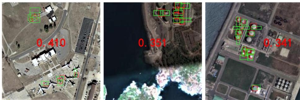
**Figure 2.** Small objects in the dataset and their corresponding positive anchors under the Faster R-CNN framework. The GT box is represented by a red rectangle, and the positive anchors corresponding to the GT box are represented by green rectangles. Numbers in the images are the average IoUs of the positive anchors corresponding to the small objects.
