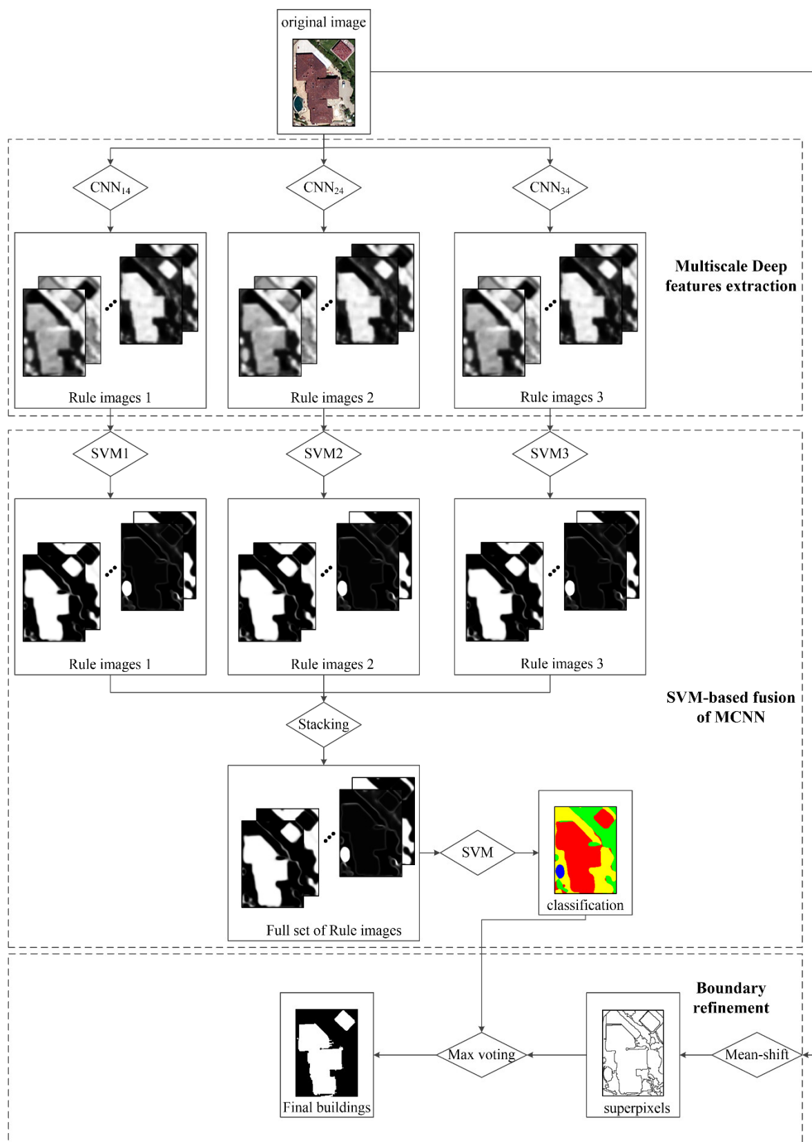
Figure 1. Framework of the proposed algorithm, which composed of three major steps: (A) Multiscale deep features extraction; (B) Support vector mechanism (SVM)-based fusion of multiscale convolutional neural network (MCNN); (C) boundary refinement. CNN_{14} , CNN_{24} , and CNN_{34} represents three CNN models with different kernel sizes.
